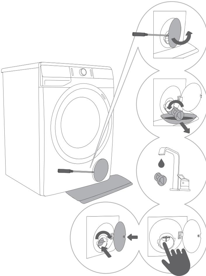
**1** Open the pump filter cap using a suitable tool (flat screwdriver or a similar tool).
