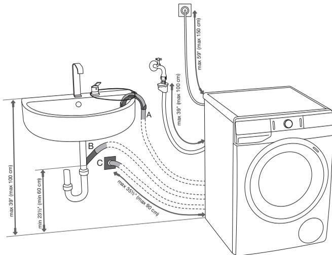
**A** Discharge hose end may be placed over a washbasin or a bathtub. B Use a string fed through the opening in the elbow support to attach the hose and prevent it from slipping to the floor.
