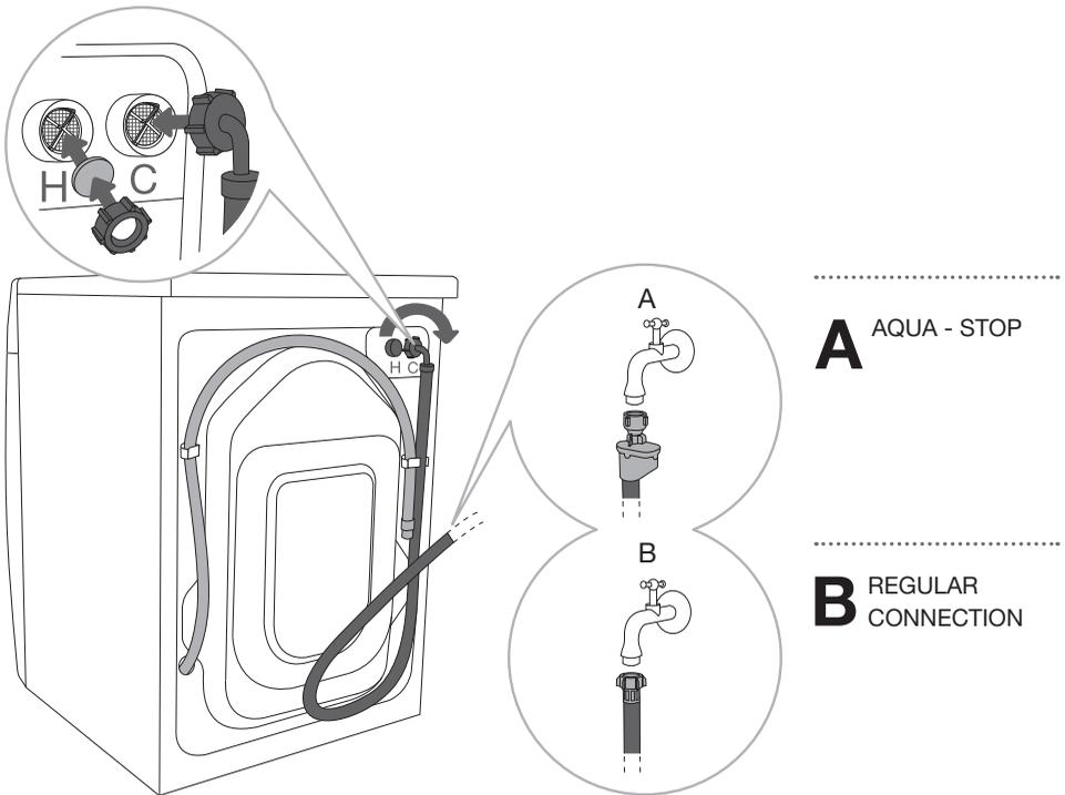
⚠ If your washing machine features a hot and cold water connection, but you only wish to connect it to cold water supply, do not install the hot water hose and close the hot water connection on the back of the washing machine with the supplied cap.
