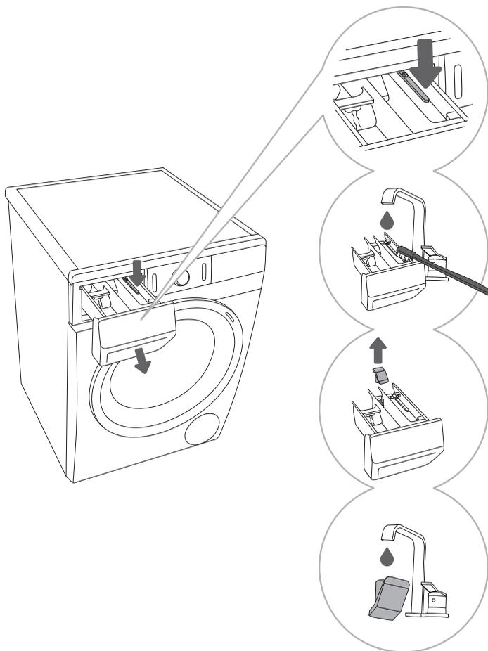
**1** To remove the dispenser tray from the housing, press the small tab.
