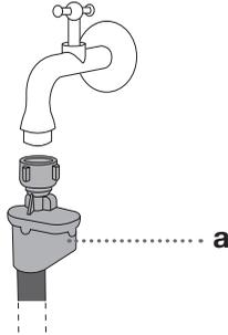
⚠ Do not dip the water supply hose with the AQUA - STOP system in water as it contains an electric valve.
