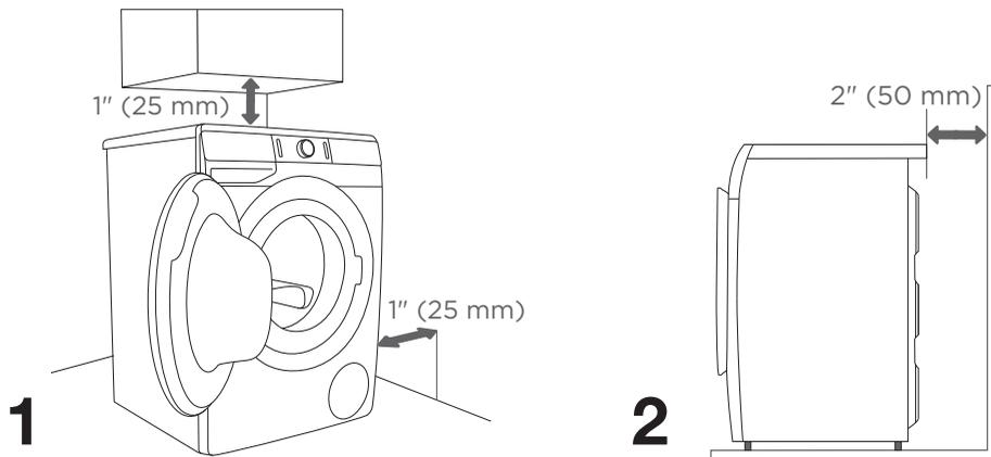
⚠ The washing machine may not be in contact with a wall or adjacent furniture. For optimum washing machine operation, we recommend observing the clearances from the walls as indicated in the figure.
