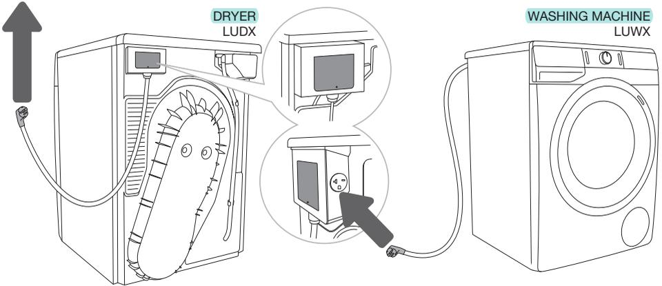
The machine is delivered ready-fitted with a plug and is intended for connection to an Dryer, which is equipped with a matching receptacle. The plug supplied with the washer can only be used with an Dryer. If the washer is used separately or with another dryer, it must be on a separate 208-240 V single-phase circuit.
