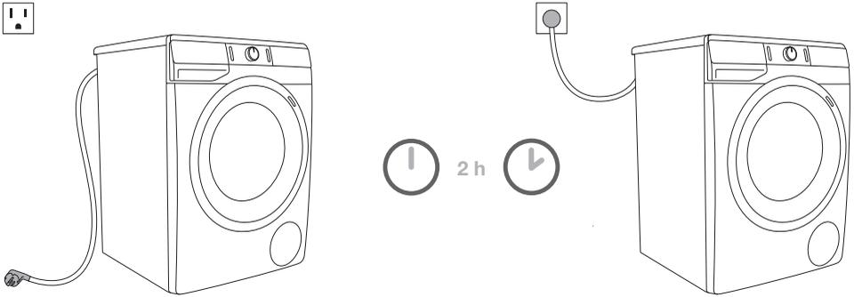
**⚠ Before connecting the washing machine to the power mains, wait for at least 2 hours until it reaches room temperature.**
