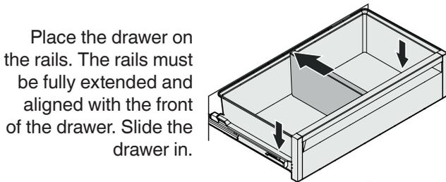
Place the drawer on the rails. The rails must be fully extended and aligned with the front of the drawer. Slide the drawer in.
