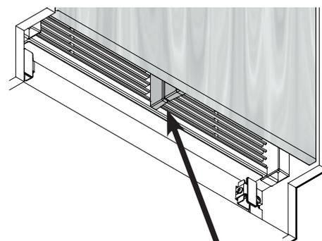
Check that there is no gap between the appliance air divider and the door air divider.
