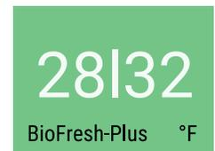
An additional drawer divider must be inserted to select 28°F / 32°F.
