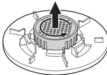
Insert the new air filter and turn clockwise until it snaps in.
