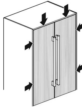
Close the doors and check the position of the door panels.
