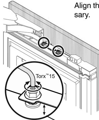
Align the panels vertically if necessary.
