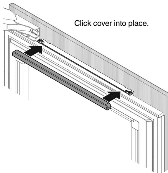
Hook the door cover strips at the front of the supports and snap in at the back.
