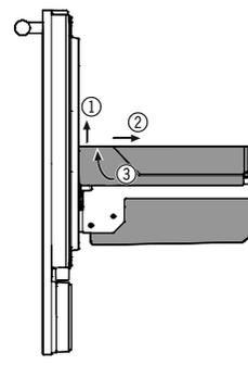
Pull the freezer drawer upwards by its right and left bottom corners (1). Push the container backwards (2). Set the container to an angle and remove it (3).
