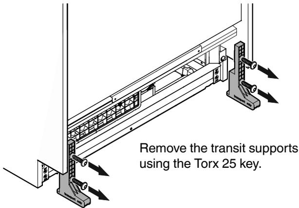
Remove the transit supports using the Torx 25 key.
