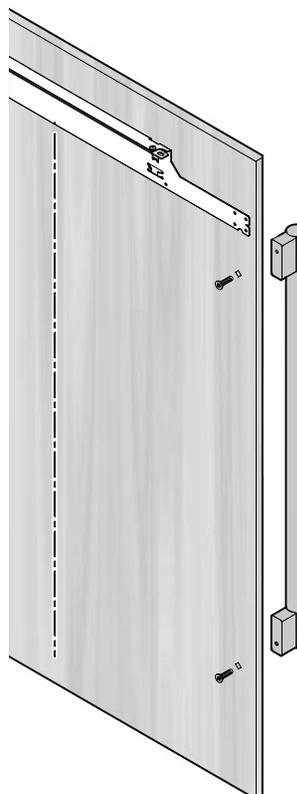
Only use countersunk screws for handle mounting.
