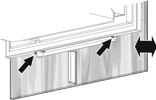
Fasten the panel through the bottom attachment bracket with two screws 4 x 14.
