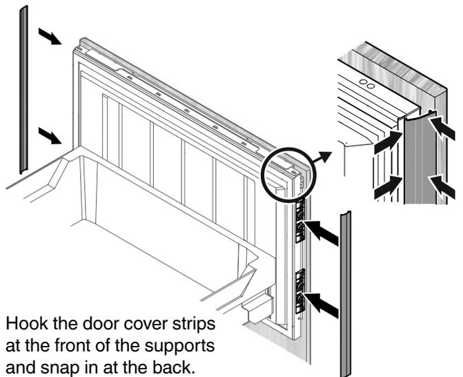
Hook the door cover strips at the front of the supports and snap in at the back.
