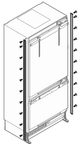
Apply the appliance cover strips to the left and right front edge of the appliance housing, align in height with the top profile and screw into place. The strip is transparent so the designed mounting holes on the appliance housing are visible. We recommend that you mark and pre-drill the hole positions in the strip.
