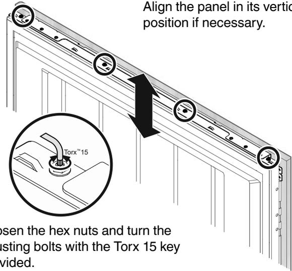
Loosen the hex nuts and turn the adjusting bolts with the Torx 15 key provided.
