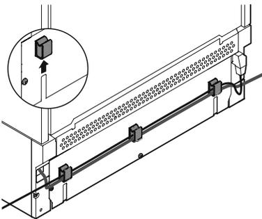
Install the cable holders on the rear of the appliance. Insert power cord/water line in cable holders.
