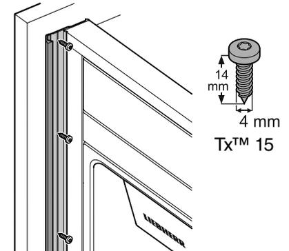
Fasten the appliance in the recess through the appliance cover strips using eight screws 4 x 14 for each side. We recommend that you mark and pre-drill the hole positions in the strip.
