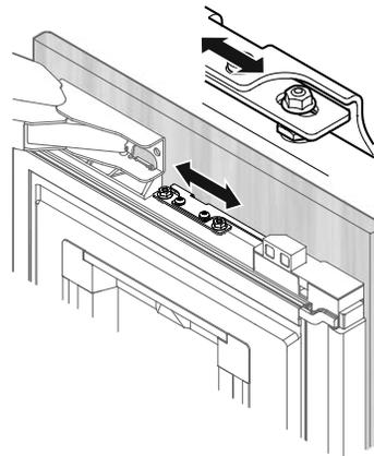
Align the panels horizontally using the long holes in the attachment bracket.
