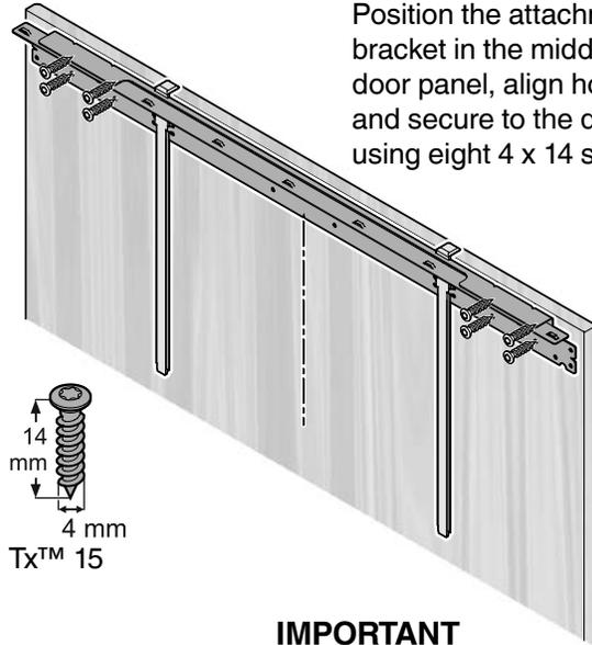
Position the attachment bracket in the middle of the door panel, align horizontally and secure to the door panel using eight 4 x 14 screws.
