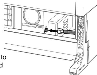
Connect the other end to the male connector and tighten.
