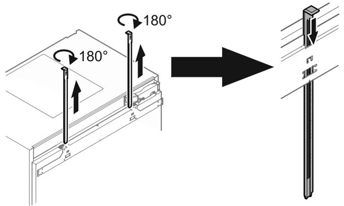
Remove the mounting strips, turn them through 180° and insert them as far as possible into the attachment bracket.
