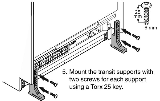
5. Mount the transit supports with two screws for each support using a Torx 25 key.
