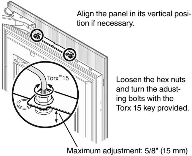
Align the panel in its depth at the bottom.
