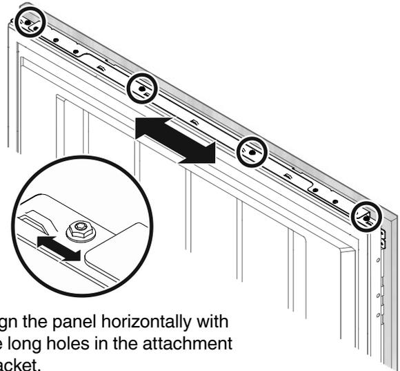
Align the panel horizontally with the long holes in the attachment bracket.
