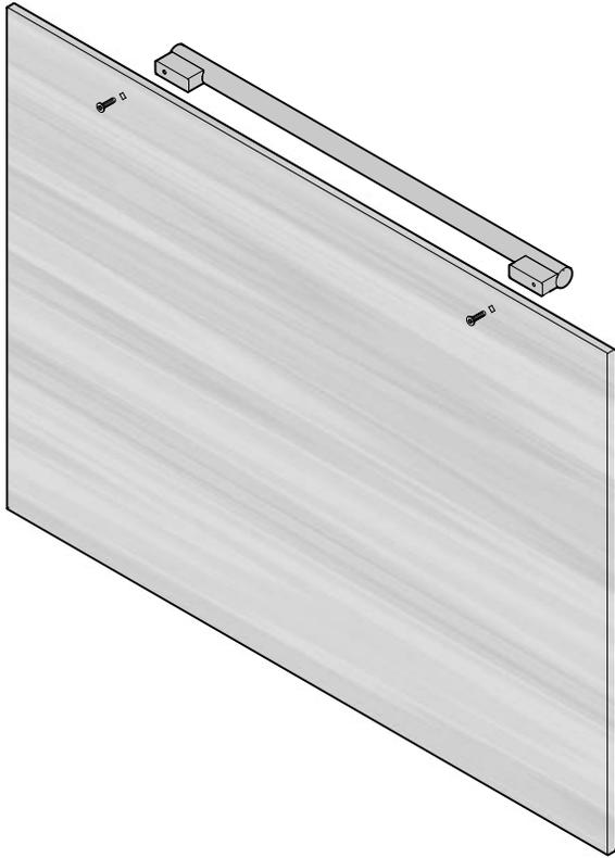
Only use countersunk screws for handle mounting.
