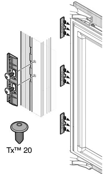
Fasten the panel through the bottom attachment bracket with two screws 4 x 14.
