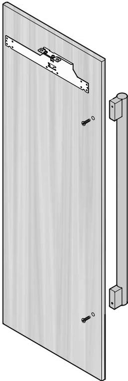
Only use countersunk screws for handle mounting.
