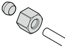
To connect to a 1/4" PEX line use a 1/4" compression nut and a plastic compression ring.
