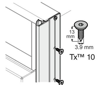
Apply the appliance cover strips to the left and right front edge of the appliance housing, align in height with the top profile and screw into place. The strip is transparent so the designed mounting holes on the appliance housing are visible. We recommend that you mark and pre-drill the hole positions in the strip.
