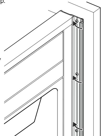
Push the mounting strip upwards. The bottom edge of the mounting strip must be aligned with the top edge of the adjacent cabinet door.
