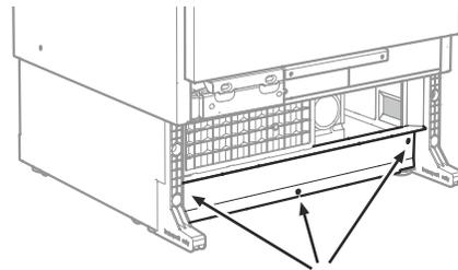
The steel plate can be removed to facilitate connecting the water hose.
