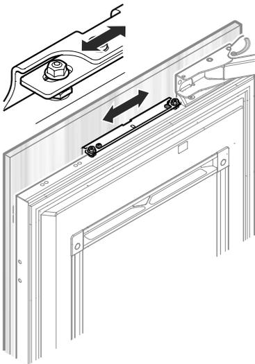
Align the panel horizontally with the long holes in the attachment bracket.
