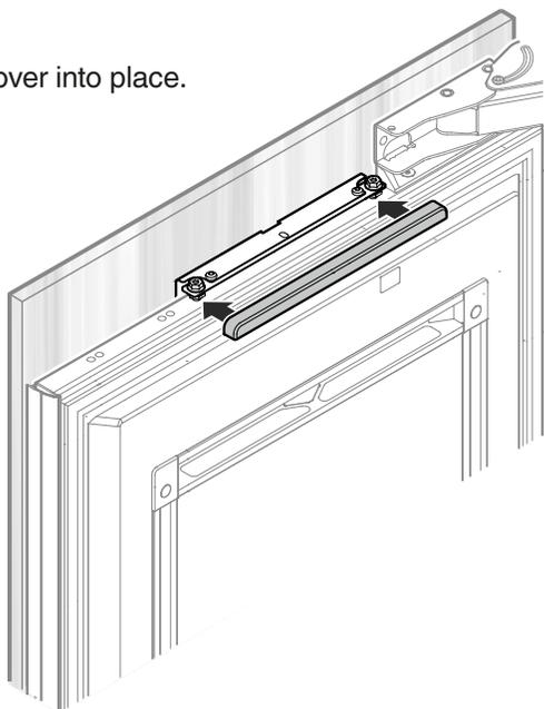
Adjust the brackets to the thickness of the toe kick panel.
