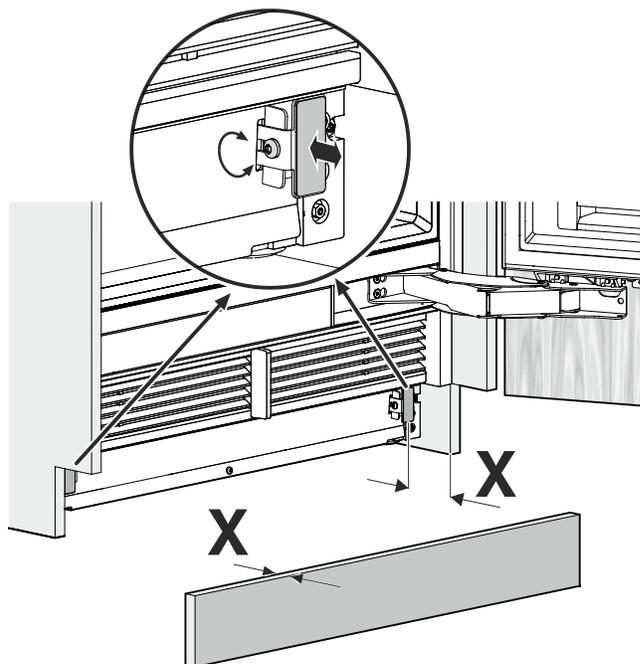
Remove the backing foil and affix the toe kick panel.
