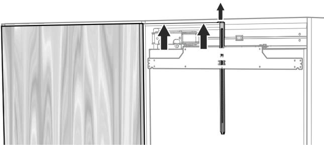
Position the attachment bracket in the middle of the door panel, align horizontally and secure to the door panel using eight 4 x 14 screws.
