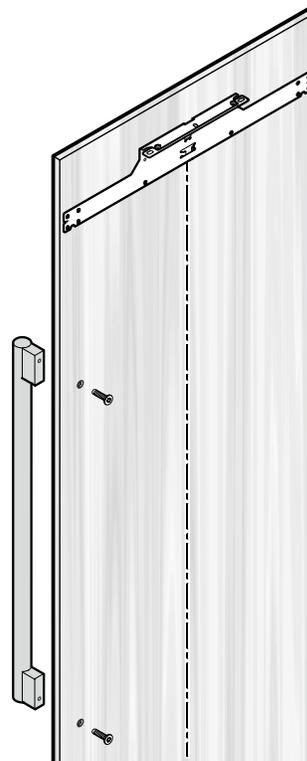
Only use countersunk screws for handle mounting.
