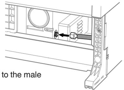
Connect the other end to the male connector and tighten.
