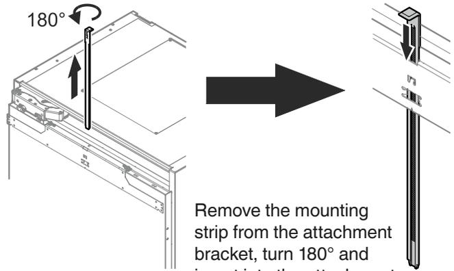
Remove the mounting strip from the attachment bracket, turn 180° and insert into the attachment bracket as far as it will go.
