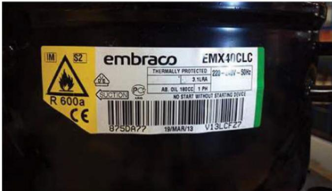
R-600a is heavier than air, do not allow any leakage/migration to low areas such as basements and stairs.
