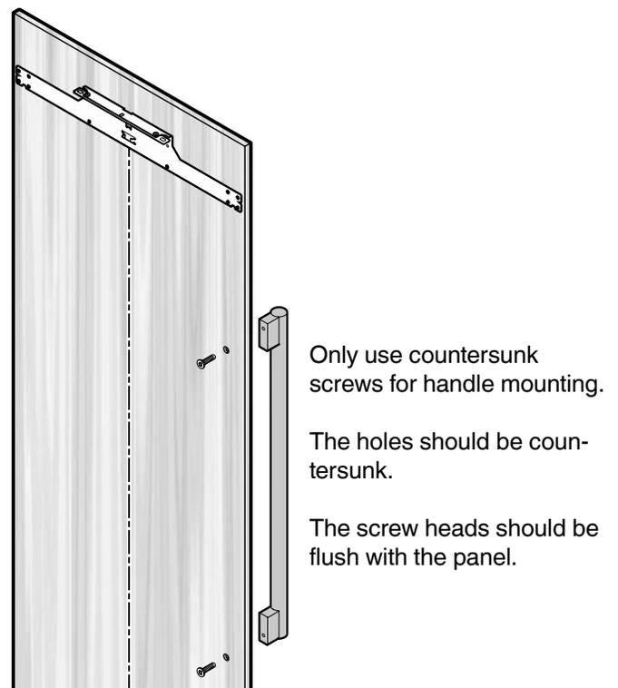
Position the panel support strips with the top lug in the cut of the top attachment bracket.
