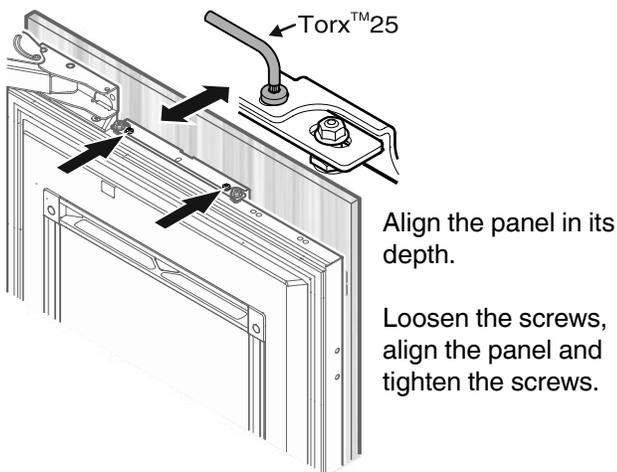
Align the panel in its depth at the bottom.
