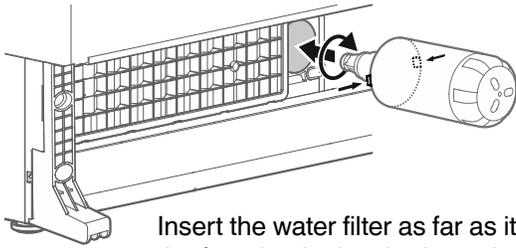
Insert the water filter as far as it will go with the front knobs in a horizontal position and turn clockwise until it snaps in.
