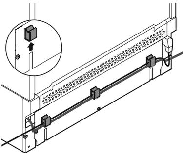
Install the cable holders on the rear of the appliance. Insert power cord/water line in cable holders.
