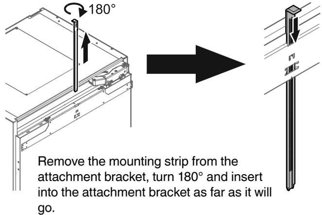
Remove the mounting strip from the attachment bracket, turn 180° and insert into the attachment bracket as far as it will go.
