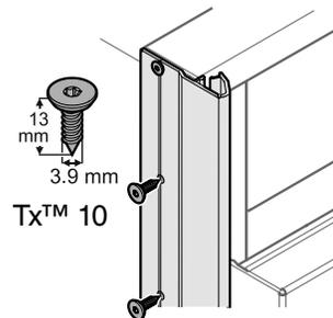
Apply the appliance cover strips to the left and right front edge of the appliance housing, align in height with the top profile and screw into place. The strip is transparent so the designed mounting holes on the appliance housing are visible. We recommend that you mark and pre-drill the hole positions in the strip.
