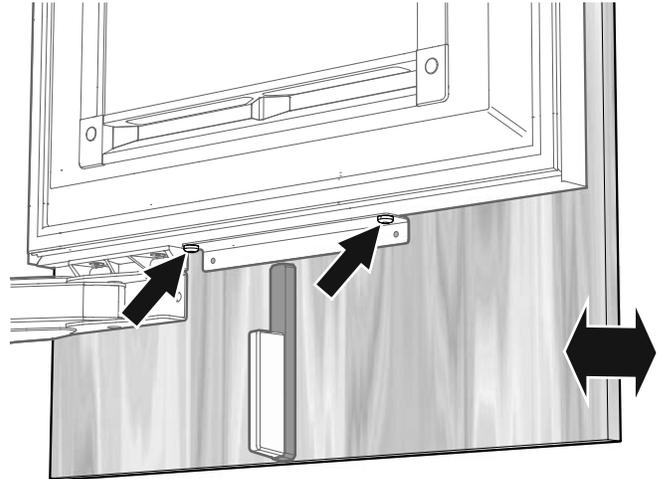
Fasten the panel through the bottom attachment bracket with two screws 4 x 14.
