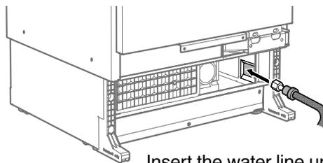
Insert the water line until it comes out on the appliance rear and pull through.
