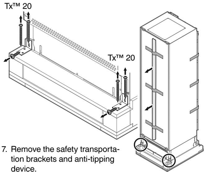
7. Remove the safety transportation brackets and anti-tipping device.
