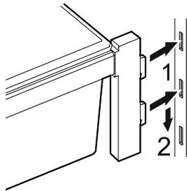
Insert the hooks of the rack into the openings of the clip-in strip at the desired height and push down.
