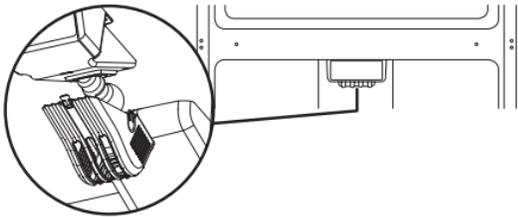
1. Remove the light shield by squeezing in on the sides and pulling it straight down.
