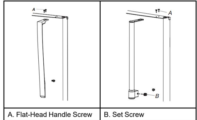
2. Remove door hinge hole plug from refrigerator door. Move to opposite side hinge hole as shown below.
