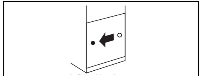
4. Remove door stop. Move to opposite side of refrigerator door as shown below.
