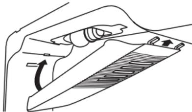
1. Remove the light shield by squeezing in on the sides and pulling it straight down.
