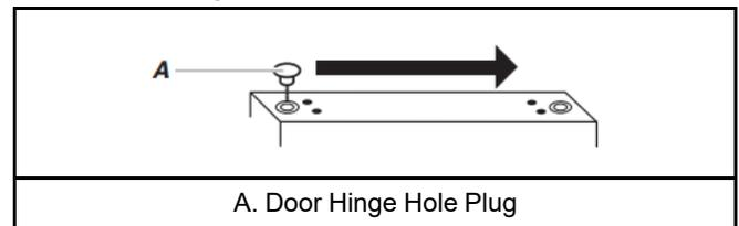
3. Remove door handle hole plug and discard. Replace on opposite side with the door handle hole plug provided in the Reversibility Kit located in the crisper.
