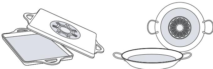
Cookware bases that contain aluminum reduce the ferromagnetic area. This may reduce the output and the cookware will not be detected sufficiently or at all, and will therefore not be heated sufficiently.
