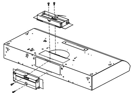
1. Using (2) short Phillips head screws, install the 3¼" x 10" (8.3 x 25.4 cm) rectangular damper over the top or rear vent knockout removed in previous step.
