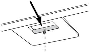
3. Remove the lateral panels by pulling them horizontally to the back of the hood and then release the brackets on the front.
