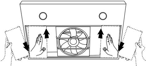
4. Using 2 or more people, lift the range hood up under cabinet and determine final location by centering beneath cabinet. Mark on the underside of cabinet the location of the 4 keyhole mounting slots on the range hood (A)
