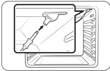
2. Insert the temperature probe plug into the socket on the top side wall of the oven.
