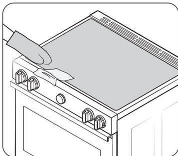
To clean the seal around the edges of the glass, lay a wet cloth on it for a few minutes, then wipe clean with a nonabrasive cleaner.
