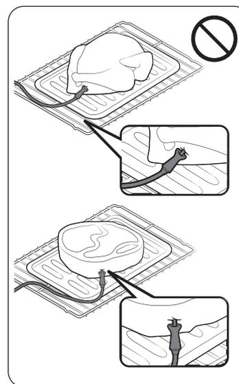
1. Push the temperature probe into the meat so that the tip of the probe reaches the center of the meat.
