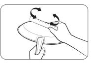
The cookware used with the cooktop surface should have flat bottoms that make good contact with the entire surface of the Cooking Zone. Check for flatness by rotating a ruler across the bottom of the cookware. Be sure to follow all the recommendations for using cookware.
