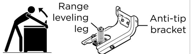
To check if the anti-tip bracket is installed properly, use both arms to grasp the rear edge of the range back. Carefully attempt to tilt range forward. When properly installed, the range should not tilt forward.
