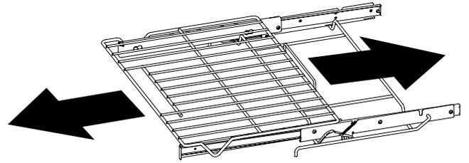
5. Turn the rack upside down and apply graphite lubrication to the insides of the loading guides.
