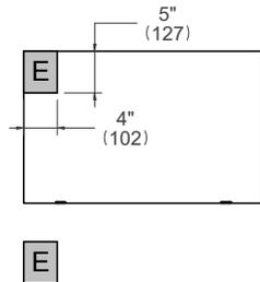
For single ovens installed into a wall cabinet, the electrical junction box may be located above, below to the left or right of the unit within reach of the power cord. Placement within the opening may require additional cabinet depth.
