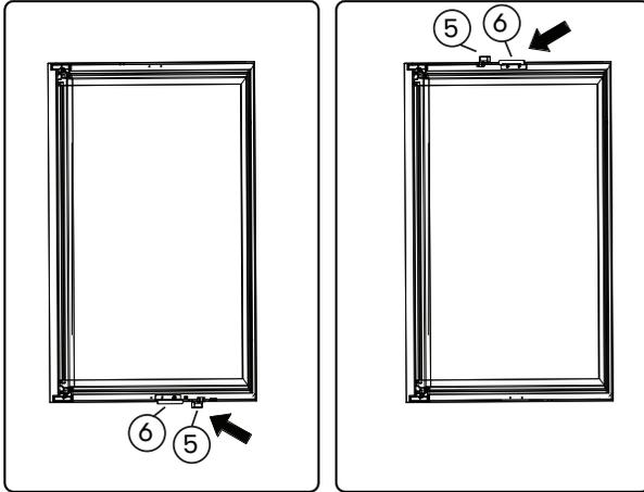
5. Remove the door magnet (5) and child safety lock catch (6) by 2 screws each and reinstall them to the opposite end of the door.
