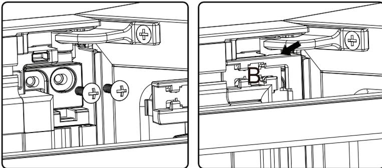
7. Once the door is aligned, tighten the 2 screws removed from step 2 at both the top and bottom corners and place the black plastic cap, marked A, to the lower left corner and the cap, marked B, to the upper left corner.
