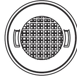
Remove the carbon filter by turning counterclockwise to unlock from rear panel.
