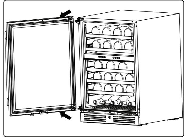
6. Mount the door over the door hinges, making sure the door magnet and child safety lock catch are both facing down.
