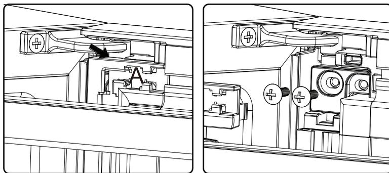
2. Remove the black plastic cap, marked A, at the upper right corner of the door and the cap, marked B, at the lower right corner. Remove 2 screws from both the upper and lower hinge.
