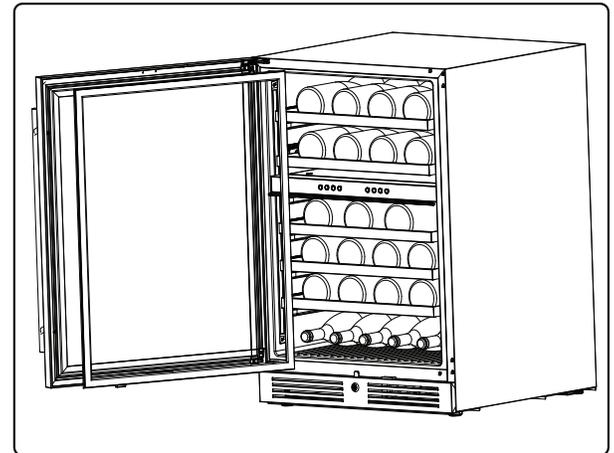
8. Reinstall the rubber door seal. Ensure the door closes tightly and there are no gaps around the seal.
