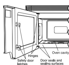
Check the oven for any damage, such as misaligned or bent door, damaged door seals and sealing surfaces, broken or loose door hinges and latches and dents inside the cavity or on the door. If there is any damage, do not operate the oven and contact your dealer or SHARP AUTHORIZED SERVICER.
