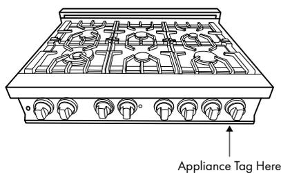
Please write down the model number and serial number of your appliance. Both numbers are located on the rating tag located under the front edge of the range top. Do not remove permanently affixed labels, warnings, or plates from the product. This will void the warranty. You may also consider attaching your receipt or proof of purchase to this manual.
