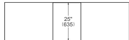
For a 25" (635) flush inset depth, max door panel thickness is 15/16" (24). Max door panel weight is 66 lbs (30 kg).
