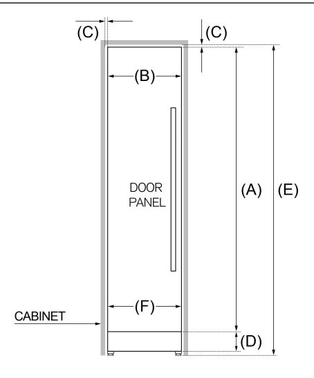
NOTE: The refrigerator comes with a 4" (100 mm) stainless steel toe kick installed to fit a standard 84" (2134 mm) tall cabinet niche.
