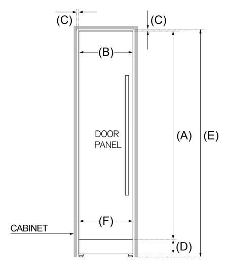
NOTE: The freezer comes with a 4" (100 mm) stainless steel toe kick installed to fit a standard 84" (2134 mm) tall cabinet niche. For flush installation in a standard 25" (635 mm) deep cabinet niche, maximum door panel thickness is 15/16" (24 mm).
