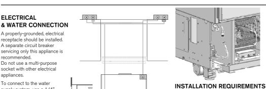
To connect to the water supply system, use a 1/4" waterline with accessible shut-off valve with a length of 60".
