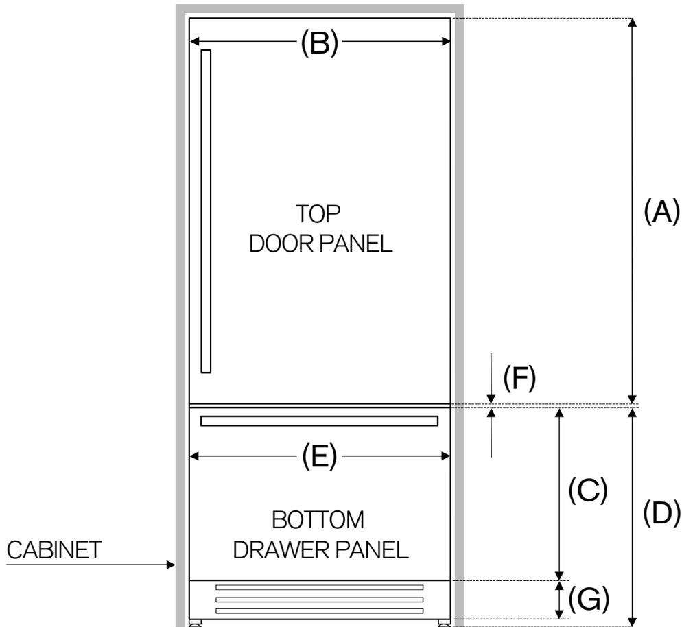
**NOTE:** These specifications assume a standard toe kick height of 4". For different toe kick heights, adjust C accordingly. C must in any case be between 21 1/2" and 25 3/4".
