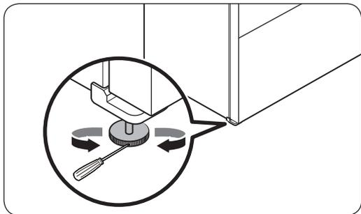
Insert a flat-head screwdriver into the leveler of the front left or right leg. Turn the leveler clockwise to raise or turn it counterclockwise to lower.
