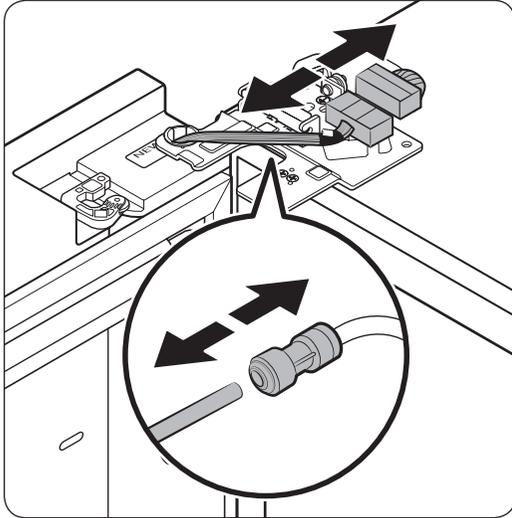
2. Disconnect the two wire connectors on the left door. The position of the connectors differs with the model.
