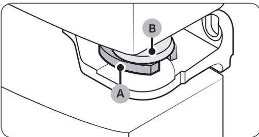
2. Insert a suitable-sized snap ring (A) between the door grommet (B) and the hinge as shown.
