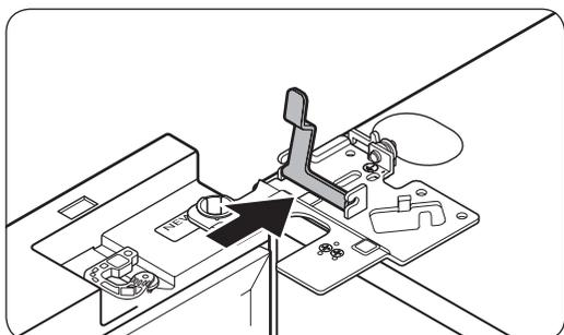
3. Insert the clamp in the direction of the arrow.
