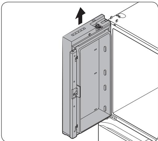
7. Gently pull up the door vertically to remove. Do not apply excessive force to the door. The door may fall, causing physical injury.
