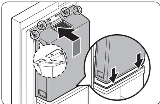
1. With the fridge door or the **Showcase door** open, align the grooves on the left and right side of the bottom door bin, and then insert it.
