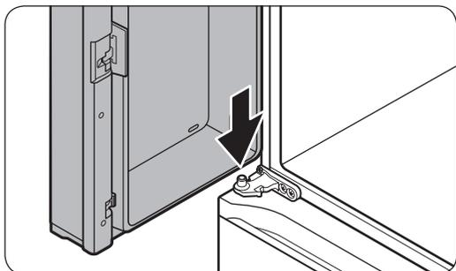
1. While holding the door open by more than 90 degrees, insert the shaft on the middle hinge into the hole on the bottom of the door.
