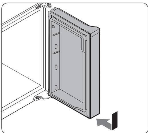
1. Insert the freezer door into the bottom hinge while pushing the freezer door in the direction of the arrow.
