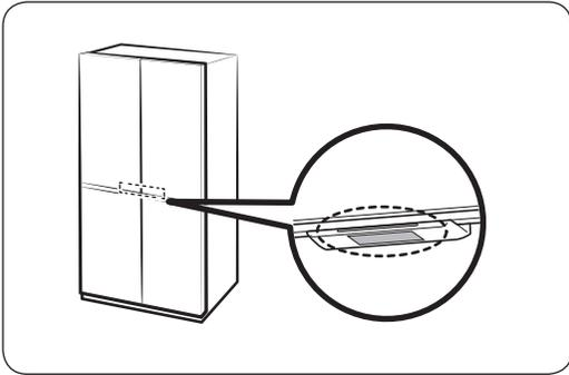
Touch the sensor near the door handle of the fridge. The door will open.
