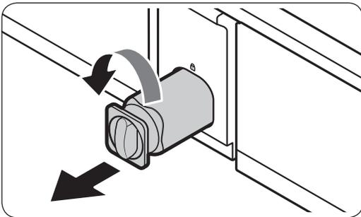
3. Turn the knob of the filter cartridge counter clockwise 90 degrees ( $\frac{1}{4}$  turn). The filter cartridge unlocks.
