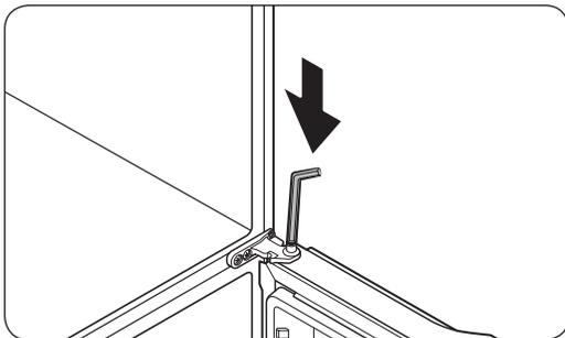
4. Locate the hinge shaft. While holding the door with one hand, use a flat-head screwdriver or Allen wrench to press the shaft down. Make sure to hold the door to prevent the door from falling.
