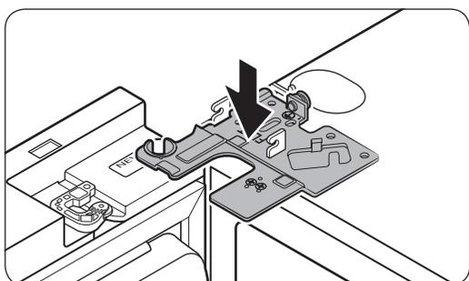
2. Put the top hinge into position on the top of the refrigerator, and then insert the hinge shaft into the top hole of the door. Make sure the wires from the door pass through the hole in the hinge shaft.
