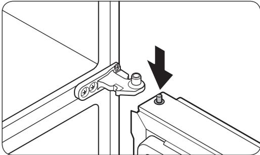
2. While pressing the hinge shaft down, position the door so that the hinge shaft is below the shaft hole in the middle hinge. Release the hinge shaft so that it enters the shaft hole.
