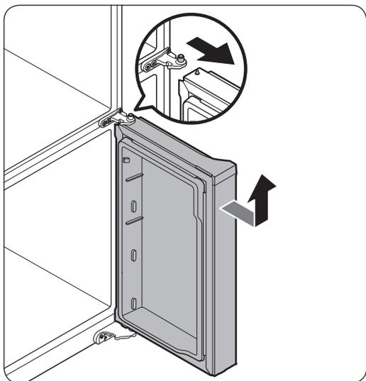
5. To prevent contact with the middle hinge, slightly tilt the door to the front, and then lift it up to remove.
