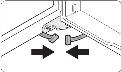
3. With the door open, connect the bottom connectors in the direction of the arrows.
