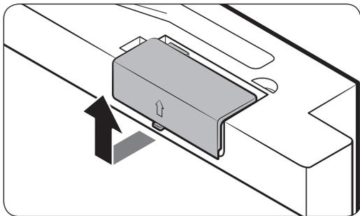
1. Open the fridge door and locate the switch cover on the top right corner of the door.
