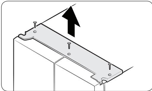
1. With the doors closed, use a Phillips screwdriver to remove the screws (x3) from the top cover. Pull up and remove the top cover with the connectors.
