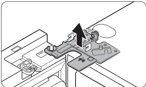
6. Open the door 90 degrees. While holding the door, pull up and remove the top hinge. Be careful not to damage the connector wires when you remove the hinge.
