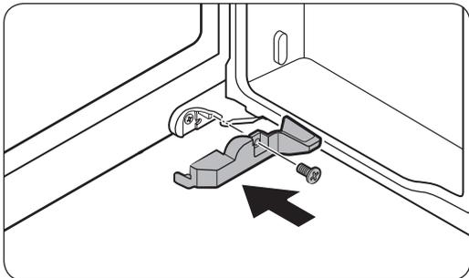
4. Attach the cover using a Phillips screwdriver. Be careful not to damage or step on the connectors.
