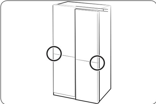
1. Check the height difference between the doors, and then lift up and hold the door with the lower height.
