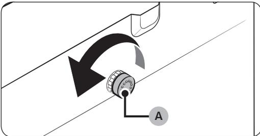
1. Open the door that is closer to the main body than the others. Then, turn the **adjustment dial (A)** counterclockwise until the gap becomes even with the others.
