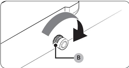
2. After adjusting the gap, turn the **locking nut (B)** to lock the **adjustment dial**.
