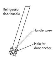
1. Screw in anchors to the door with a Phillips-head screwdriver.
