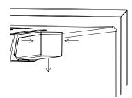
1. When the refrigerator is used for the first time, press down on the marks on both sides of the filter cover by hand (see above), and move the filter cover downward.
