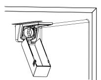
Rotate the water filter bypass plug counterclockwise and remove (see above). Please
