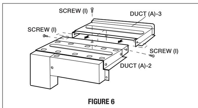
E. Remove SCREWS from the upper right and left corners at the rear of the oven. Place duct assembly on the top of the unit as shown and secure the duct assembly to the oven using the 2 SCREWS just removed from the oven. See Figure 6B.
