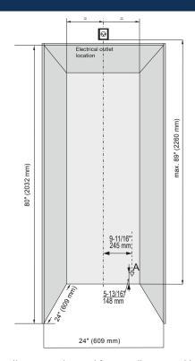
The appliances can be used freestanding or semi built-in. If semi built-in, consider the minimum cabinet opening dimensions specified on this image.
