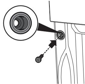
4. Cover the bushings with the covers removed previously.
