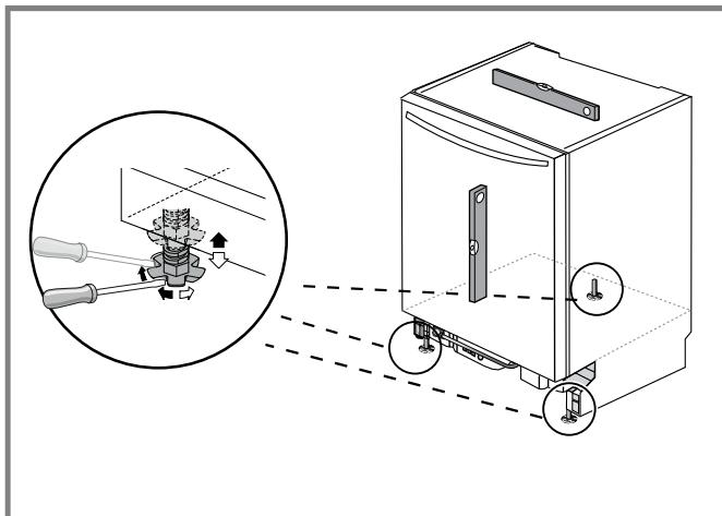
The maximum height the unit can be raised to is 34.5" (867.3 mm)
