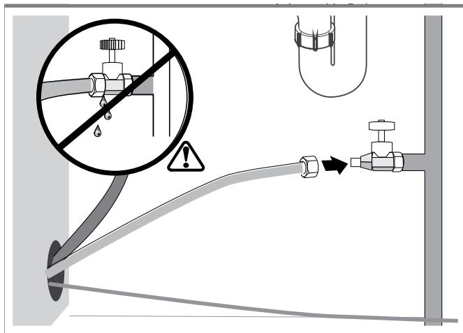
**3** Properly tighten all water connections.
