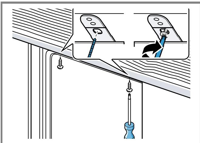
If the dishwasher came with a protective barrier, screw through the barrier.
