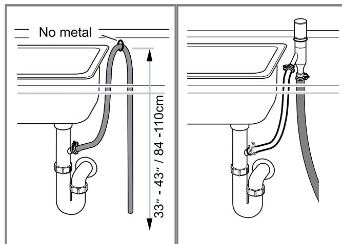
4. Tighten the hose clamp around the house plumbing.
