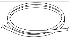
Water inlet hose - minimum 3/8" outer diameter copper tubing or metal braided dishwasher supply line.
