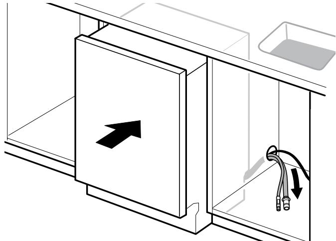
5. Reach into adjacent cabinet and pull hoses and excess power cord completely out so they do not get kinked.
