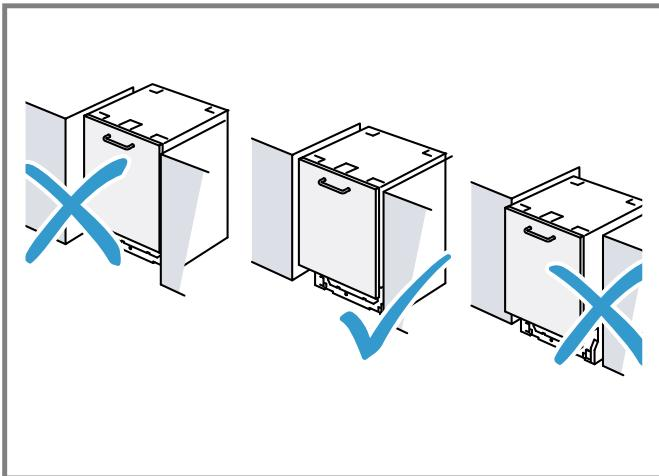
3. Make sure the top of the door is no less than 1/4" (6mm) from the underside of the counter.
