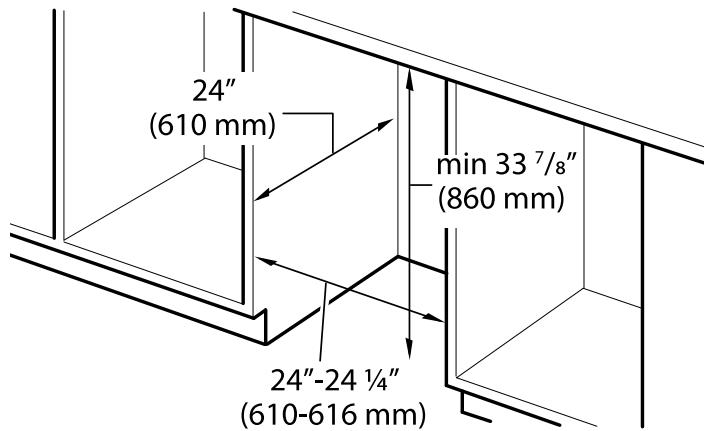
If the dishwasher is to be installed in a corner, ensure that there is adequate clearance to open the door as shown.
