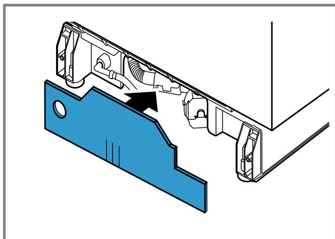
3. Attach the toe panel with the 3/4" screws so it is flush with the floor. Use black screws for a black toe panel and stainless for a white toe panel.
