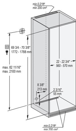
This is a fully integrated refrigerator-freezer appliance designed to be completely enclosed in a dedicated kitchen cabinet. This dedicated cabinet box must be constructed in accordance with the specified dimensions and must allow for sufficient air circulation to ensure proper operation.
