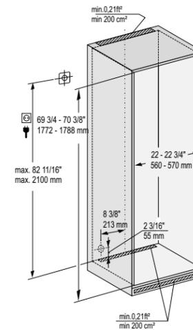
This is a fully integrated wine appliance designed to be completely enclosed in a dedicated kitchen cabinet. This dedicated cabinet box must be constructed in accordance with the specified dimensions and must allow for sufficient air circulation to ensure proper operation. For more details about ventilation requirements, please refer to page 44.
