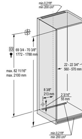
This is a fully integrated refrigerator-freezer appliance designed to be completely enclosed in a dedicated kitchen cabinet. This dedicated cabinet box must be constructed in accordance with the specified dimensions and must allow for sufficient air circulation to ensure proper operation. For more details about ventilation requirements, please refer to page 44.
