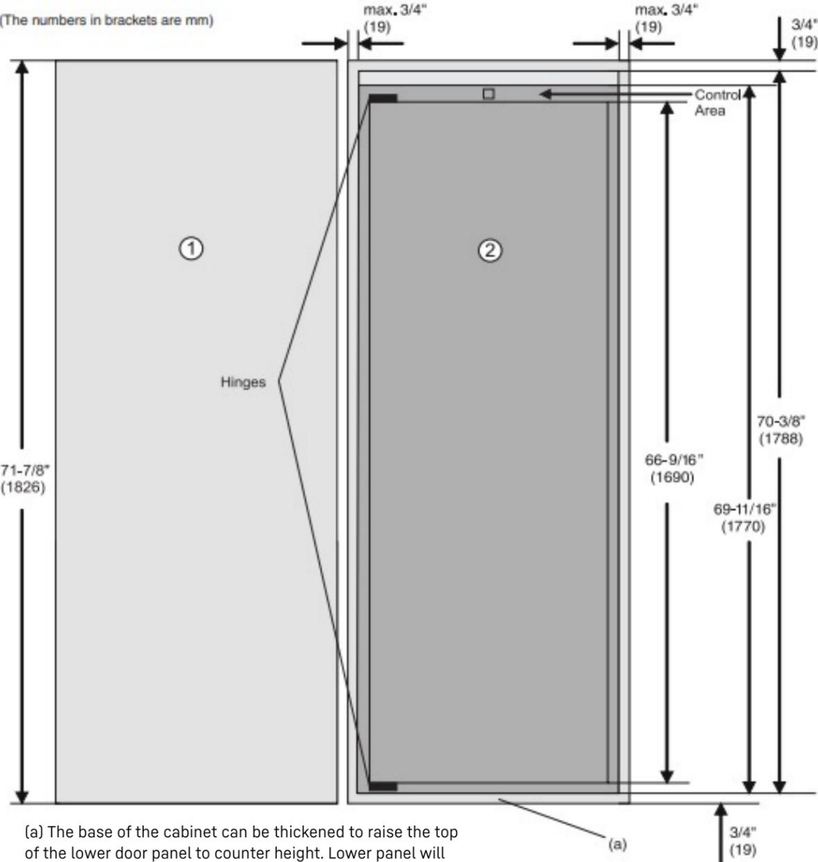
(a) The base of the cabinet can be thickened to raise the top of the lower door panel to counter height. Lower panel will have to be increased in length by the same amount.
