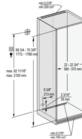
This is a fully integrated refrigerator appliance designed to be completely enclosed in a dedicated kitchen cabinet. This dedicated cabinet box must be constructed in accordance with the specified dimensions and must allow for sufficient air circulation to ensure proper operation. For more details about ventilation requirements, please refer to page 44.
