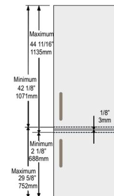
This is a sliding door model, which means the doors of the appliance are installed on the hinges of the dedicated box cabinet doors.
