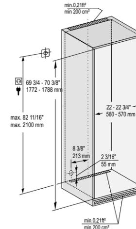
This is a fully integrated refrigerator-freezer appliance designed to be completely enclosed in a dedicated kitchen cabinet. This dedicated cabinet box must be constructed in accordance with the specified dimensions and must allow for sufficient air circulation to ensure proper operation. For more details about ventilation requirements, please refer to page 44.
