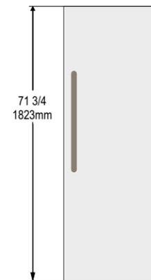
Custom panels should be at least 5/8" (16mm) and a maximum of 3/4" (19mm) thick and they should cover the front of the dedicated cabinet box.
