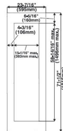
Custom panels should be at least 5/8" (16mm) and a maximum of 3/4" (19mm) thick and they should cover the front of the dedicated cabinet box.
