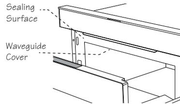
**2** Remove the feature sticker, if there is one. Check the drawer for any damage, such as misaligned or bent drawer, damaged drawer seals and sealing surfaces, broken or loose drawer guides and dents inside the cavity or on the front side of the drawer. If there is any damage, do not operate the Microwave Drawer and contact your dealer or a SHARP AUTHORIZED SERVICER.
