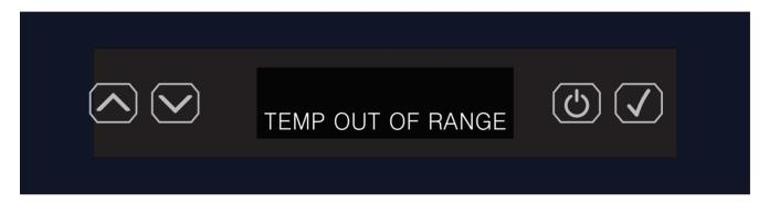
The TEMP OUT OF RANGE alert activates when the temperature level is out of range by 10 degrees Fahrenheit for a 12-hour time period.
