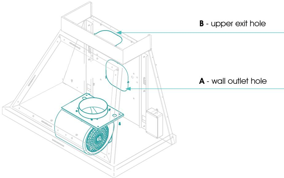
rotate the motor and fix
