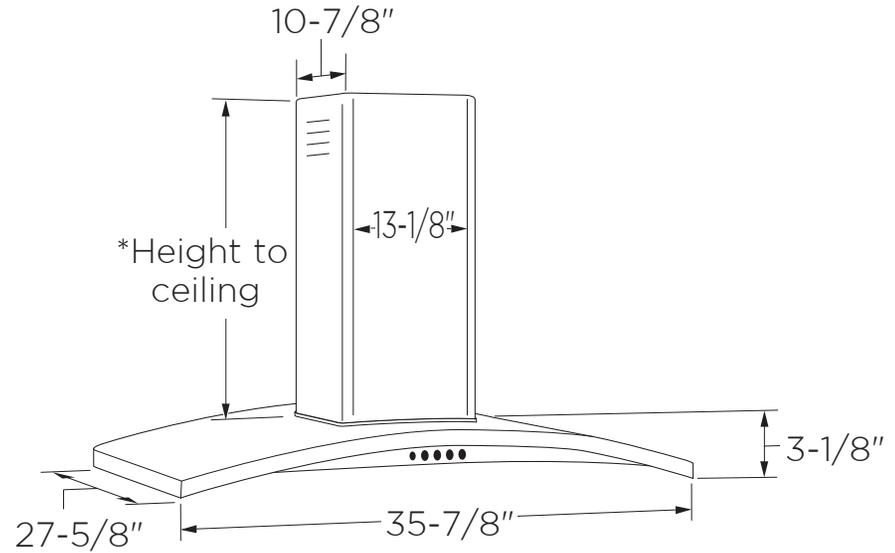
\*The supplied duct cover fits 7'11" to 10'4" ceiling heights (10'9" in recirculation mode).
