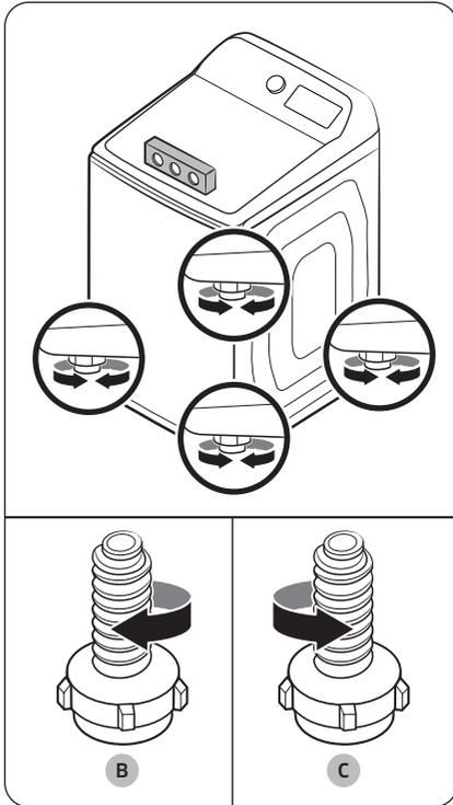
4. If the washer is not level, turn the appropriate leveling feet **clockwise (B)** to lower the washer, or **counterclockwise (C)** to raise the washer so that it is level.
