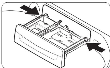
2. To remove, pull the detergent drawer while pushing the ends of each side in.
