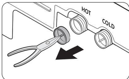
4. Use pliers to pull out the mesh filter from the inlet valves.
