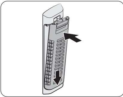
3. When cleaning is complete, close the cover and reinsert the filter case to the original position. You will hear a clicking sound when the filter case fits in.
