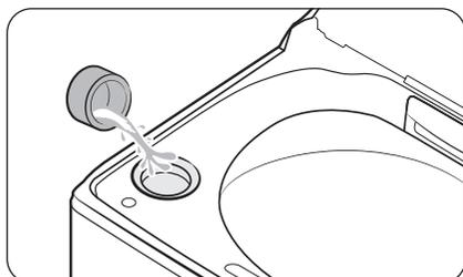
Add only liquid chlorine bleach to the bleach compartment. Do not exceed the max line.
