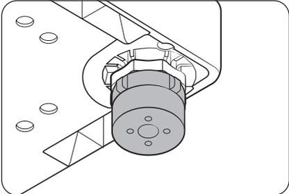
With the leg ring in place, use the leveling leg to adjust the height of the washer.
