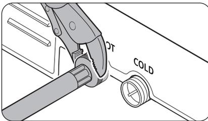
4. Attach the water hoses to the hot and cold water inlets on the back of the washer, and then hand tighten the water hose fittings until they are tight. Then, use pliers to tighten the fittings by an additional two-thirds of a turn.
