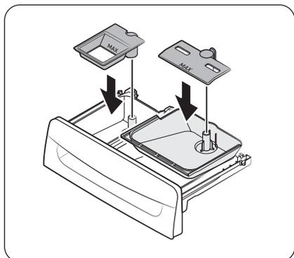
3. Remove the inserts from the compartments. Rinse the inserts and the drawer in warm water and clean with a soft brush.
