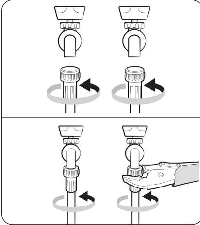
1. Attach the water hoses to the hot and cold water taps, and then hand tighten the water hose fittings until they are tight. Then, use pliers to tighten the fittings by an additional two-thirds of a turn. To avoid damaging the fittings, do not overtighten them.
