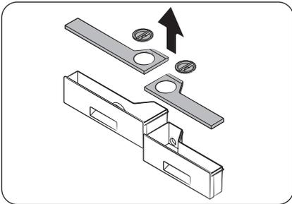
3. Remove the lids of both dispensers using the pull tabs at the back of each lid.
