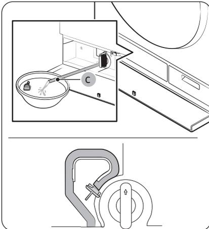
5. Open the tube cap and let water in the **emergency drain tube (C)** flow into the container.
