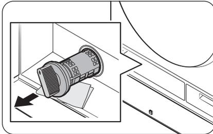
5. Turn the drain filter knob to the left, and drain off the remaining water.
