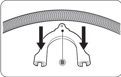
2. Attach the drain hose to the **plastic hose guide (B)**.
