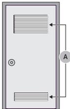
**A:** If the Laundry Combo is installed in the same location with other washer or dryer, the front of the alcove or closet must have two unobstructed air openings for a combined minimum total area of 72 in.<sup>2</sup> (465 cm<sup>2</sup>).
