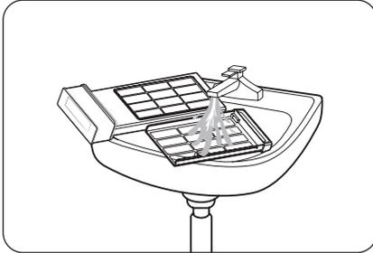
4. Remove lint on both inner and outer filters. Then, wash the filters in running water and completely dry the filters in a shade.
