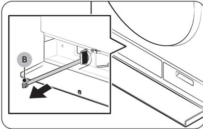
4. Put an empty, spacious container around the cover, and stretch the emergency drain tube to the container while holding the **tube cap (B)**.
