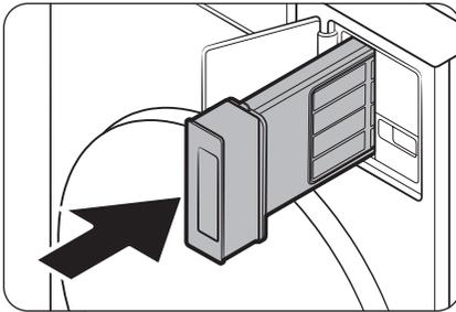
5. Put the inner filter into the outer filter in the correct direction.
