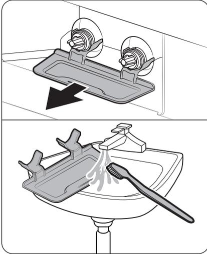
5. Remove the dispenser tray and clean it in running water to remove leaked detergent or softener. Then, put the tray back.
