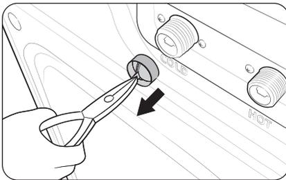
4. Use pliers to pull out the mesh filter from the inlet valve.
