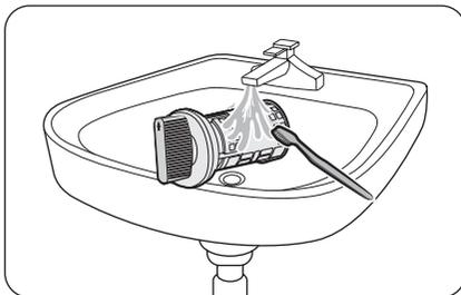
6. Clean the drain filter using a soft brush. While the drain filter is removed, make sure the impeller inside the drain pump is free of debris.
