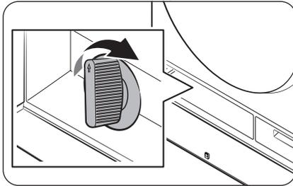
7. Reinsert the drain filter, and turn the filter knob to the right.
