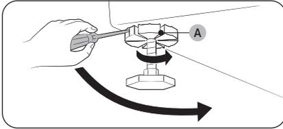
3. Using a flathead screwdriver, tighten the **locking nuts (A)**.
