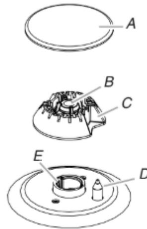
A. Burner cap      D. Igniter electrode
