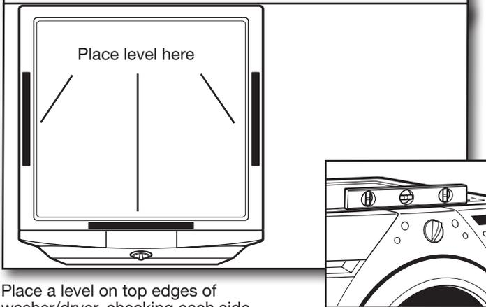
Place a level on top edges of washer/dryer, checking each side and front. Rock washer/dryer back and forth to make sure all four feet make solid contact with floor.
