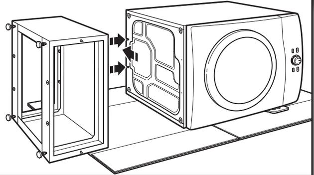
Move the pedestal against the dryer bottom. The front of the pedestal cabinet should align with the dryer cabinet as shown below.
