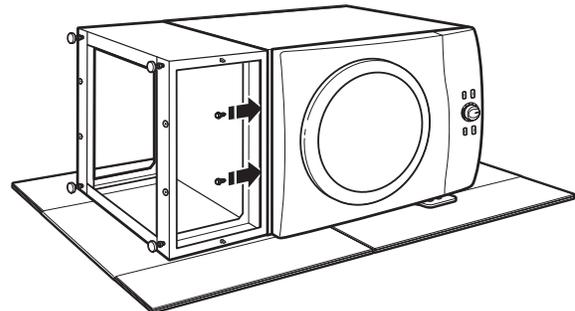
Position the pedestal toward the front of the dryer and install the two remaining hex-head sheet metal screws. Do not tighten completely. Now proceed to "Complete the pedestal installation".
