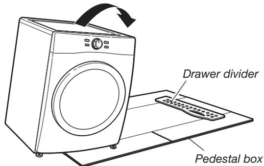
To avoid floor damage and ease installation and handling, unfold the empty pedestal box flat and place it next to the dryer. Position the drawer divider so that it will be near the top of the dryer, as shown. Gently tip the dryer on its side so the dryer is resting on the drawer divider.
