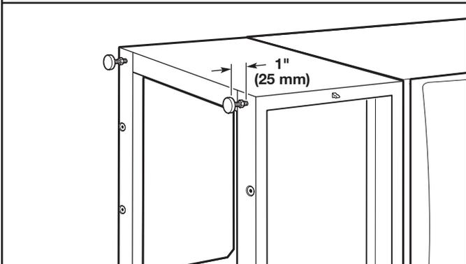
Using a 1/4" hex head ratchet or open-end wrench, lower the feet approximately 1" (25 mm) away from the bottom of the pedestal.
