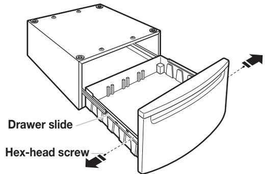
Using a 1/4" nut driver, remove the hex-head screws from both drawer slides and save screws. Remove the drawer from the slides and set aside. Push the slides back into the pedestal.
