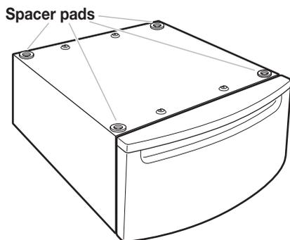
The four spacer pads are installed on the top of the pedestal. These pads reduce vibration between the pedestal and the washer/dryer.
