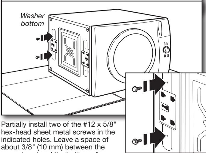
Partially install two of the #12 x 5/8" hex-head sheet metal screws in the indicated holes. Leave a space of about 3/8" (10 mm) between the screw head and the bottom of the washer.
