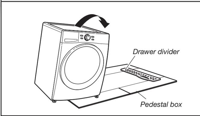
To avoid floor damage and ease installation and handling, unfold the empty pedestal box flat and place it next to the washer. Position the drawer divider so that it will be near the top of the washer, as shown. Gently tip the washer on its side so the washer is resting on the drawer divider.
