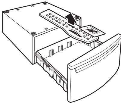
Open the pedestal drawer as far as possible and remove the contents. The package contains four #12 x 5/8" hex-head sheet metal screws and a drawer divider.
