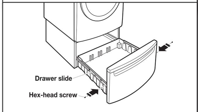
Pull both drawer slides out and reassemble the drawer to the drawer slides with the two hex-head screws.
