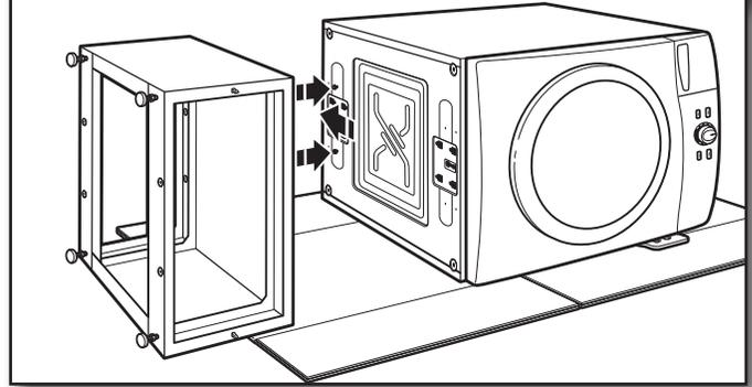
Move the pedestal against the washer bottom. The front of the pedestal cabinet should align with the washer cabinet as shown below.
