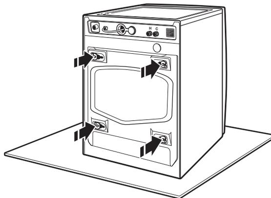
Locate the transport bolts on rear of washer. Transport bolts must remain in washer before pedestal can be installed. For more information on transport bolts see, "Remove Transport System" in washer Use and Care Guide.
