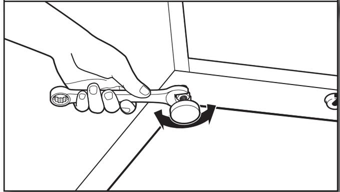
When the washer/dryer is level, use a 9/16" open-end wrench to securely tighten all four jam nuts against the pedestal.
