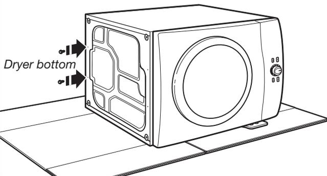
Partially install two of the #12 x 5/8" hex-head sheet metal screws in the indicated holes. Leave a space of about 3/8" (10 mm) between the screw head and the bottom of the dryer.
