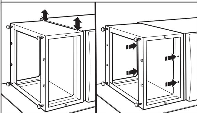
Align the sides of the pedestal so that they are even with the sides of the washer/dryer. Reach inside the pedestal opening and securely tighten all four pedestal screws.
