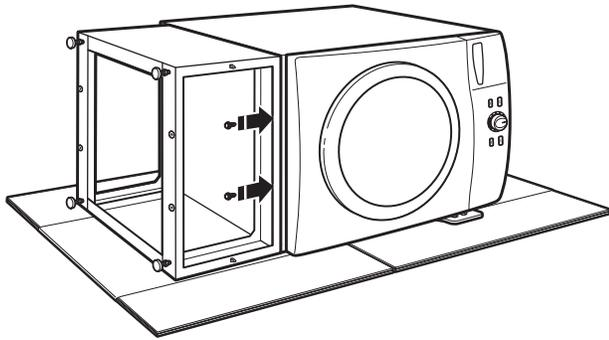
Position the pedestal toward the front of the washer and install the two remaining hex-head sheet metal screws. Do not tighten completely. Now proceed to "Complete the pedestal installation".
