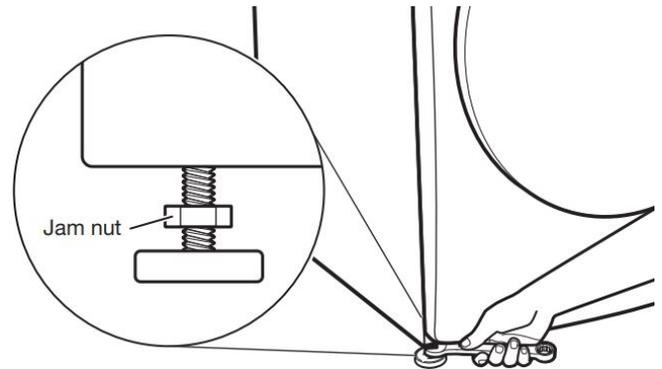
If washer is not level, use a 9/16" (14.3 mm) open-end or adjustable wrench to turn jam nuts clockwise on feet until they are about 1/2" (13 mm) from the washer cabinet. Then turn the leveling foot clockwise to lower the washer or counterclockwise to raise the washer. Do not exceed 2" (50 mm) from bottom of foot to bottom of cabinet. Recheck levelness of washer and that all four feet are firmly in contact with the floor. Repeat as needed.
