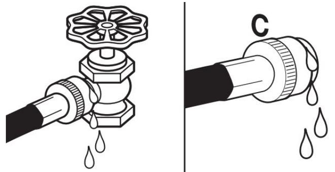
Slowly turn on water faucets to check for leaks. A small amount of water may enter washer. It will drain later.
