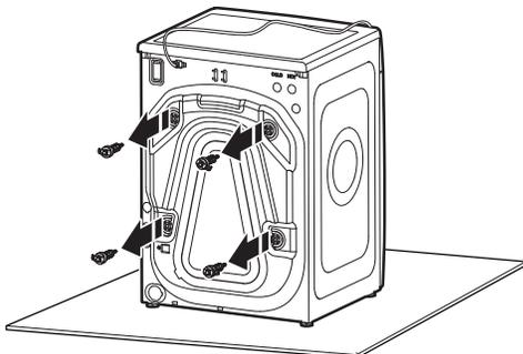
Loosen bolts with a 5/8" (16 mm) wrench. Slide each bolt and spacer to center of hole. Pull bolts and plastic spacers from back of washer. Discard bolts and spacers.
