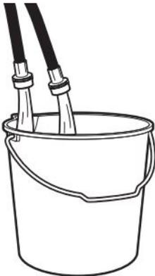
Run water for a few seconds through hoses into a laundry tub, drainpipe, or bucket to avoid clogs. Water should run until clear.
