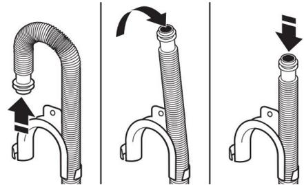
For floor drain installations, you will need to remove the drain hose form from the end of the drain hose. You may need additional parts with separate directions; refer to the Quick Start Guide.
