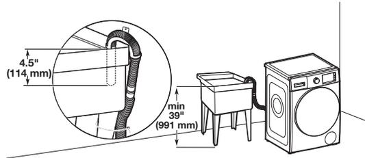
Minimum capacity: 20 gallons (76 L). Top of laundry tub must be at least 39" (991 mm) from the floor; install no higher than 48" (1.2 m) from bottom of washer.
