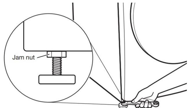
When washer is level and all four feet are firmly in contact with the floor, use a 9/16" (14.3 mm) open-end or adjustable wrench to turn jam nuts counterclockwise on leveling feet tightly against washer cabinet.
