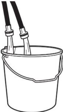
Run water for a few seconds through hoses into a laundry tub, drainpipe, or bucket to avoid clogs. Water should run until clear.
