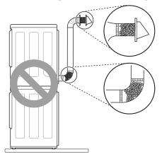
Make sure the ductwork is not crushed or restricted.
