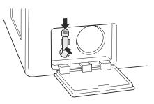
7 Insert the drain pump filter and twist it clockwise.
