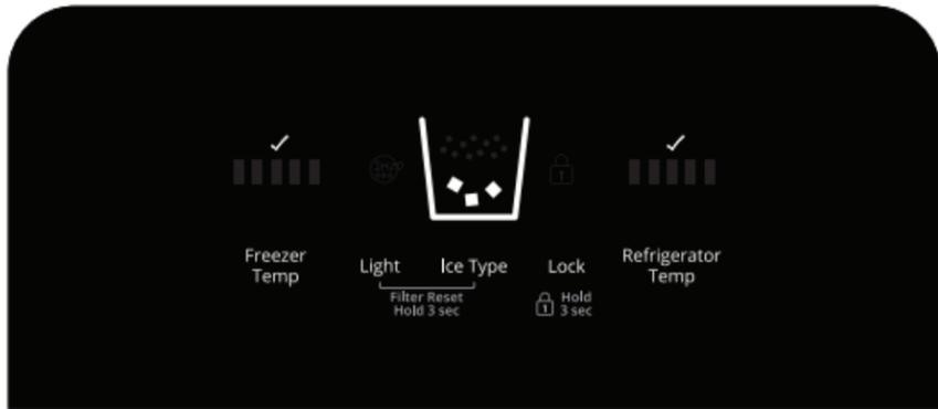
For your convenience, your refrigerator and freezer controls are preset at the factory. When you first install your refrigerator, make sure that the both the refrigerator and freezer controls are still set to the "mid-setting." This will be indicated with three illuminated bars.
