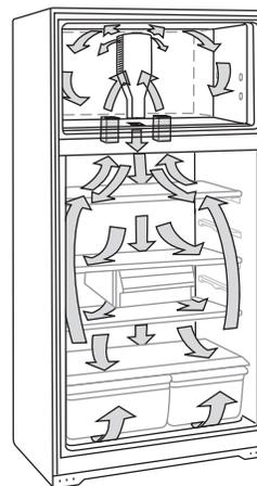
Do not block any of these vents with food packages. If the vents are blocked, airflow will be restricted and temperature and moisture problems may occur.
