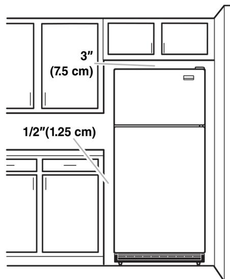
To ensure proper ventilation for your refrigerator, it is recommended to allow a 1/2" (1.25 cm) space on each side and between overhead cabinets and refrigerator top. Allow at least 1" (2.54 cm) between back of cabinet and the wall. If your refrigerator has an ice maker, make sure you leave extra space at the back for the water line connections.
