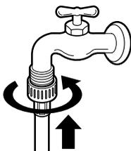
**3** After the hoses are connected, turn on the water faucets and flush out any foreign substances such as dirt, sand, or sawdust. Foreign substances can damage washer inlets and lead to leakage.
