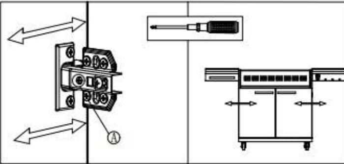
**To adjust the gap between the door and the frame - turn Screw B on the hinges.**
