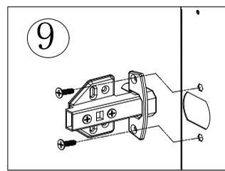
**Attach the Left Door / Hinge Assembly to the Cart Left Side #12 with 8 - M4x12 screws. Attach the Right Door / Hinge Assembly to the Cart Right Side #24 with 8 - M4x12 screws.**
