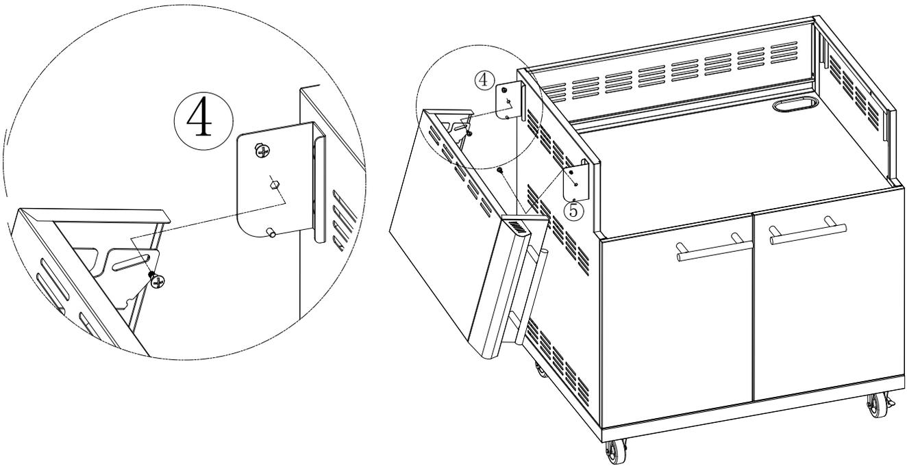
**To attach the Right Side Shelf Front #(20) to the Right Side Shelf #(21), turn both parts upside down. Start, but do not tighten down 2 - M5x10 bolts as shown below into the Right Side Shelf Front #(20). Align the heads of the bolts with the keyhole slots in the Right Side Shelf #(21) and slide into place to align both parts. Install the additional 3 - M5x10 bolts as shown and tighten all 5 bolts.**
