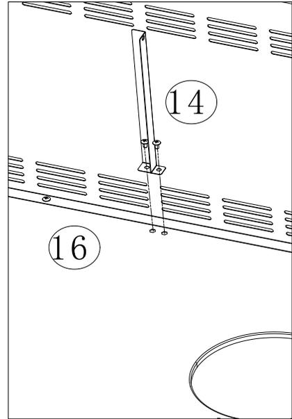
**Install the Front Panel Support #(15) to the Bottom Panel #(16) with 2 - M5x10**
