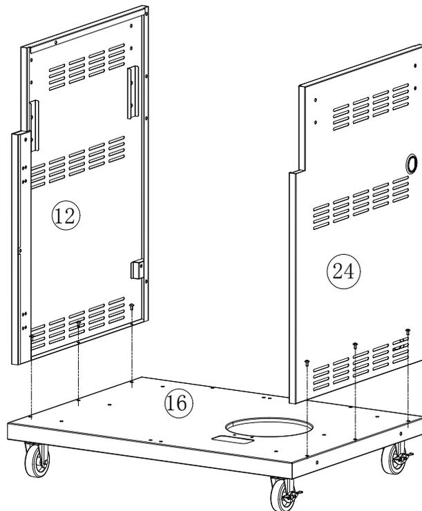
**Place the Cart Rear Lower Panel # (2) between the Left # (12) and Right # (24) Side Panels. Use 6 - M5x10 bolts to fasten to the sides and the base.**
