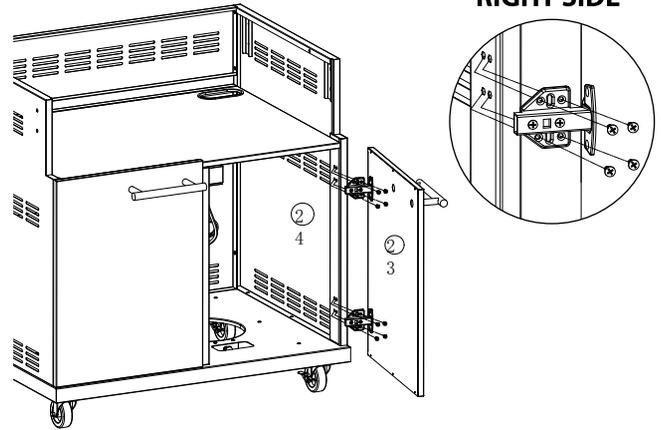
**To adjust the gap between the doors - turn Screw A on the hinges.**
