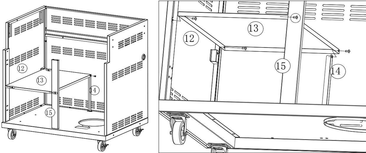
**Attach the Top Panel # (3) to the Left Side Panel # (12), Front Panel Support # (15), Cart Rear Upper Panel # (1) and Right Side Panel # (24) with 6 - M5x10 bolts**
