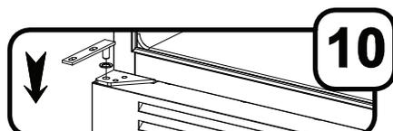
**Step 10:** Install the lower hinge pin and washer.
