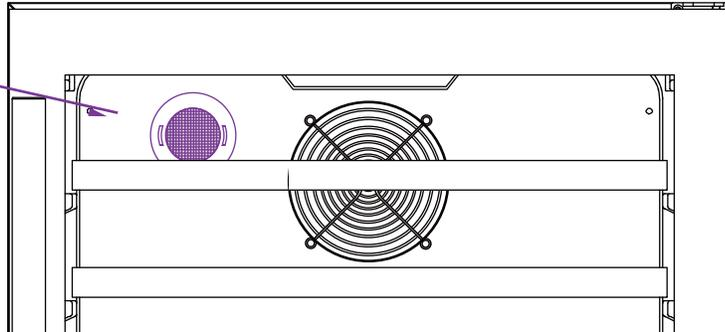
Rotate the filter 1/4 turn to unlock
