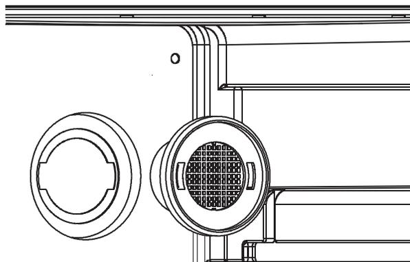
Rotate filter 1/4 turn to lock in place
