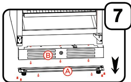
**Step 7:** Remove the front leveling leg support (A) - this will expose the screws (below and behind) holding the toe kick in place. Remove the toe kick (B).
