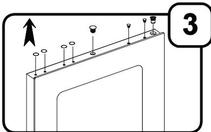
**Step 3:** Lay the door on a secure, flat, padded, working surface. **USE CARE NOT TO DAMAGE THE FINISH OR DOOR GASKET** Remove and save the plugs, stickers and hardware from the top of the door.
