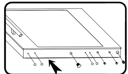
**Step 5:** Reinstall the hardware from the bottom of the door removed in **Step 4** in the holes provided in what had previously been the top of the door.
