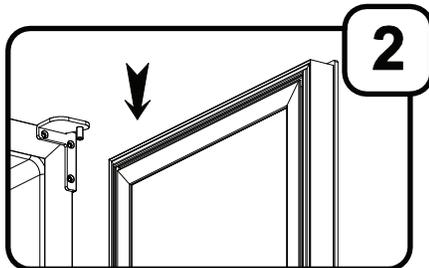
**Step 2:** Swing the bottom hinge out of the way and carefully slide the door free from the top hinge pin.
