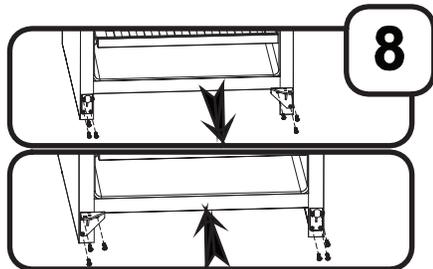
**Step 8:** Remove the lower hinge support and door bracket as shown. Reinstall the door bracket on the opposite side and install the new opposite facing lower hinge support in its place.
