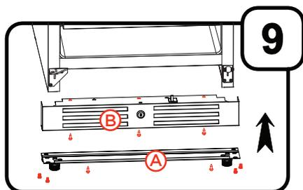
**Step 9:** First, replace the toe kick (B) removed in Step 7, then replace the front leveling leg support (A) removed in Step 7.
