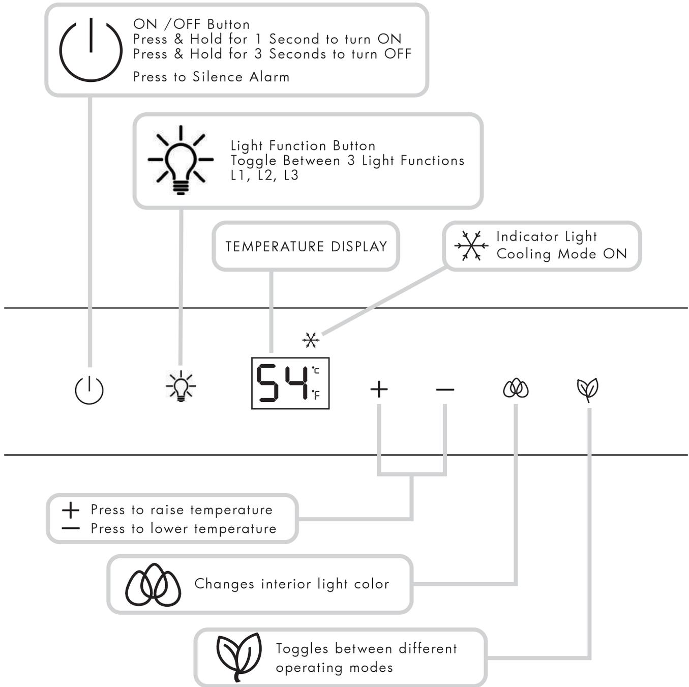
The temperature setting can be adjusted from 41-64°F. Your controls are simple and intuitive to operate.
