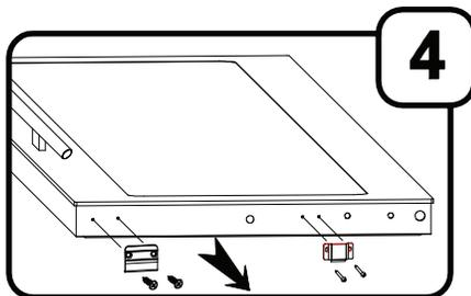
**Step 4:** Remove the hardware from the bottom of the door and replace it with the parts removed in **Step 3**.
