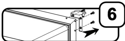
**Step 6:** Remove the upper hinge on the cabinet and replace it with the opposite facing upper hinge, supplied.
