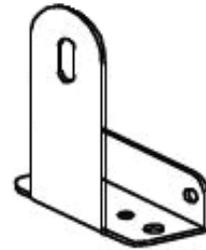
The Anti-Tip Bracket kit comes with a bolt and washers to mount to the rear of the refrigerator and three different sets of fasteners to mount it to any of the following: Dry Wall Construction, Wooden Flooring or Concrete Flooring.
