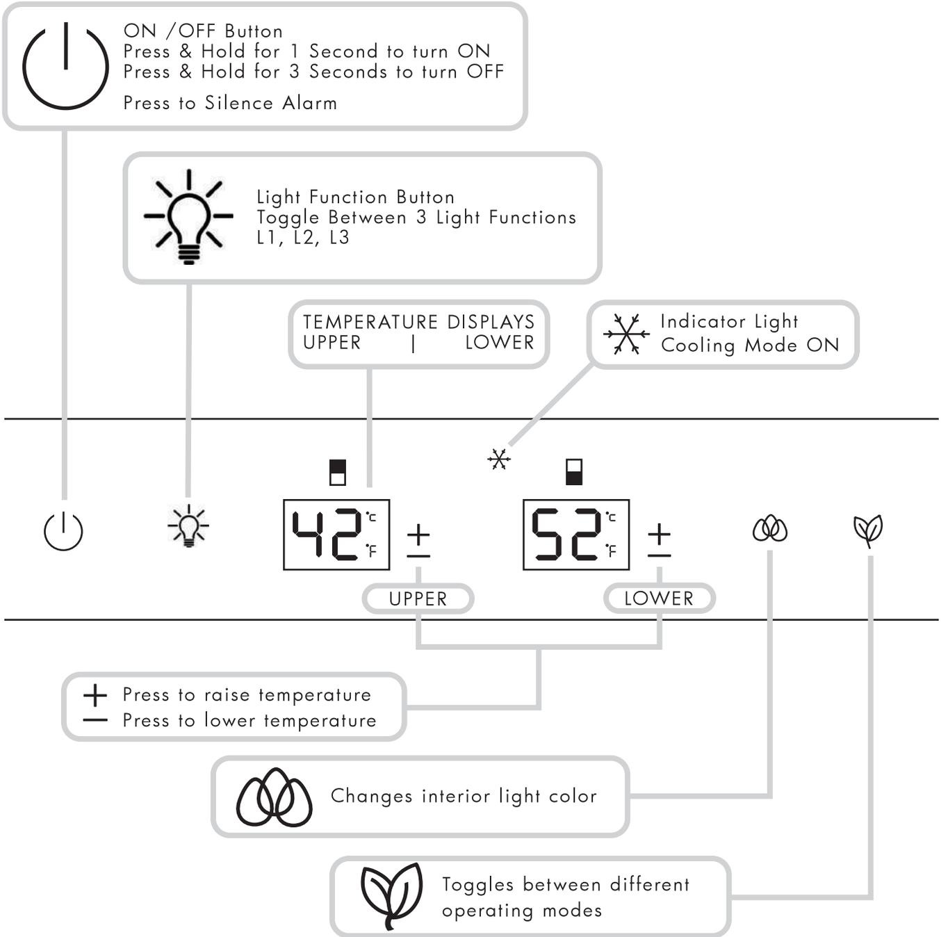
Upper compartment: The temperature setting can be adjusted from 41-50°F.
