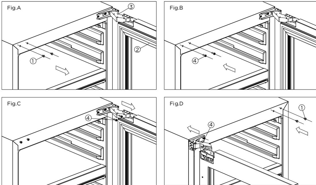
1. Screw hole covers      2. Door      3.Hinge      4.Screws
