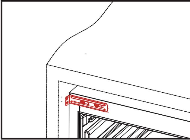
With the door open, using the screws provided connect the tie in bracket in the upper corner of the wine cooler opposite the hinge - then screw the flange of the bracket to the cabinet.
