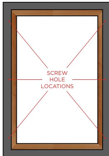
Mounting screw holes are located in the gasket channel behind the gasket.
