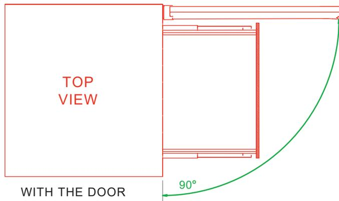
WITH THE DOOR OPEN AT 90° THE UNIT HAS A DEPTH OF 46 1/16" (1170mm)
