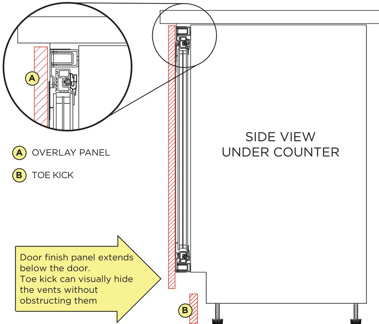
The XOU24 GOA series is 32 1/4" Tall. The standard US undercounter refrigerator is 34" Tall. Allow the additional panel length to extend as an apron below the door. The panel extension and toe kick are now able to visually hide the vents without obstructing air flow.
