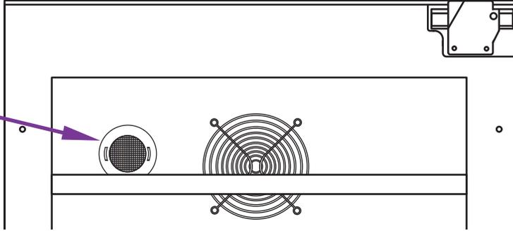
Rotate the filter 1/4 turn to unlock
