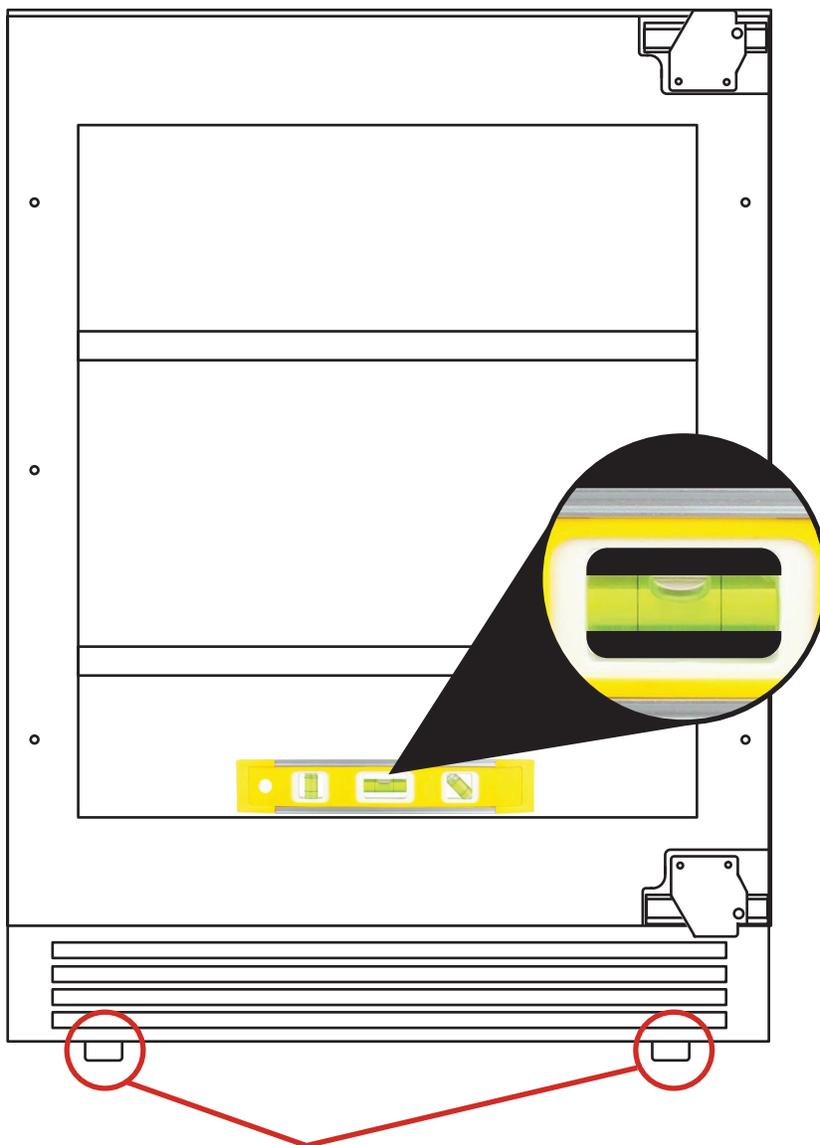
Rotate to raise or lower the **LEVELING LEGS** located at each of the four corners until all four legs are seated firmly on the floor and the interior floor of the unit is level **both front to back and side to side**.
