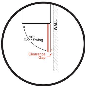
INSTALLING NEXT TO A WALL, ENSURE ADEQUATE CLEARANCE FOR THE HANDLE
