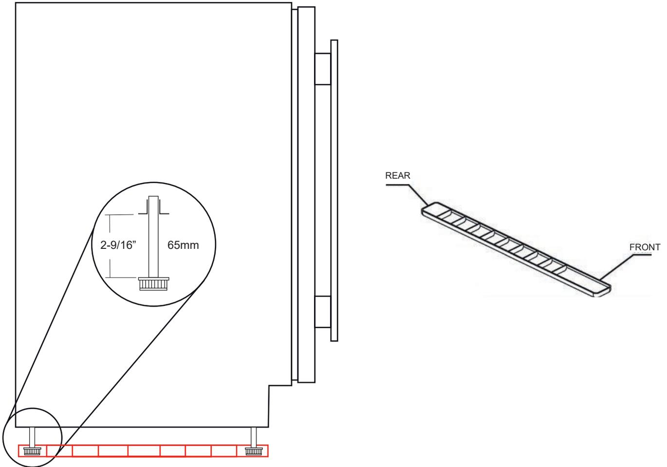
To compensate for different height cabinetry, your XO has leveling legs that can extend as much as 2-9/16" (65mm).
