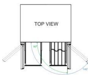
WHEN INSTALLING WITH THE HINGE SIDE NEXT TO A WALL, LEAVE ENOUGH CLEARANCE GAP FOR CABINET HANDLES. DOOR MUST BE ABLE TO OPEN A MINIMUM OF 90° FOR THE SHELVES AND RACKS TO EXTEND.
