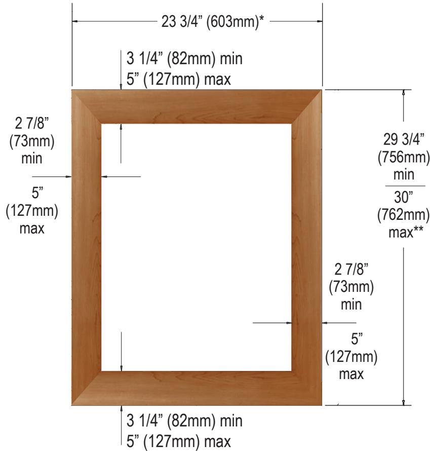
\* IF FRAME WIDTH EXCEEDS 23 3/4" WHEN MOUNTING TO THE DOOR ALIGN THE FRAME EVEN WITH THE HINGE SIDE, LETTING THE EXCESS OVERHANG THE HANDLE SIDE TO AVOID INTERFERENCE WITH THE ZERO CLEARANCE HINGE.
