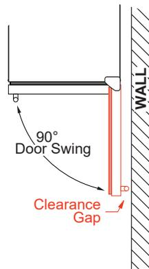
WHEN INSTALLING WITH THE HINGE SIDE NEXT TO A WALL - LEAVE ADEQUATE SPACE FOR CABINET HANDLES
