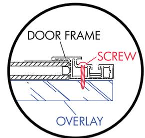
6. Align the frame to the door. If the frame is wider than the door,
