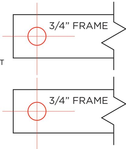
TO ACCOMMODATE THE HINGE PINS ON THE HINGE SIDE OF THE PANEL Drill a hole at least 5/16" in diameter and 1" deep into the top and bottom of the frame in the location shown.
