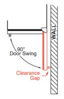
WHEN INSTALLING WITH THE HINGE SIDE NEXT TO A WALL -
