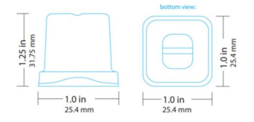
The XOUIM1565S series ice maker produces large cube gourmet ice that is crystal clear ideal for use in all kinds of beverages. That's because the rectangular bell shaped cubes are designed to melt slowly and minimize any dilution. The spray molding process allows impurities that can add taste or odor to be continuously washed away. It is ice created for the purist in you.
